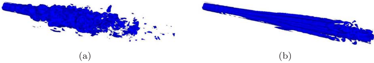
Figure 4.7: The vorticity of an LES of a jet at Re = 2,000 (a) with and (b) without disturbances of the mean velocity flow at the inlet.
