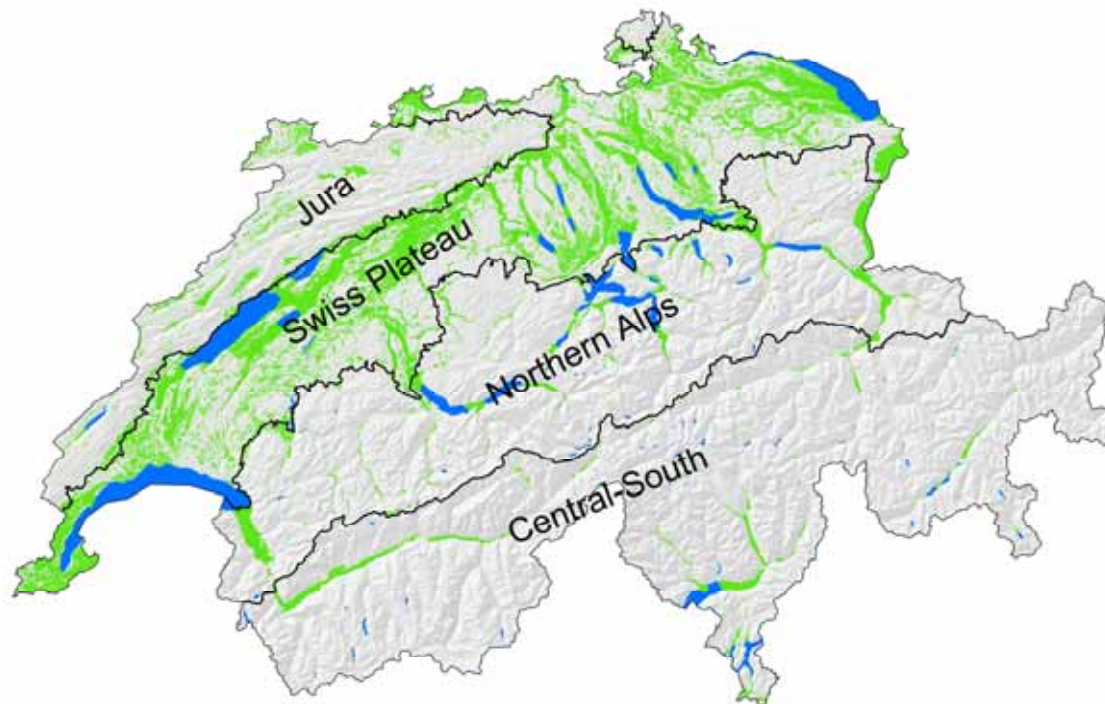
Fig. 2.2.2: Results of the simple flood model yielding potentially flooded areas. The model uses a potentially natural stream network based on a Digital Elevation Model. The green areas represent the simulated potential wetlands along larger rivers.
