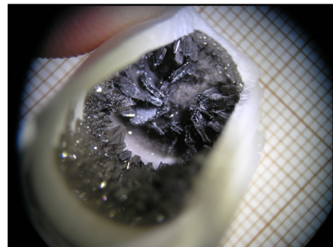
Fig. 6. Spontaneous growth of GaN crystals in the BN crucible.
