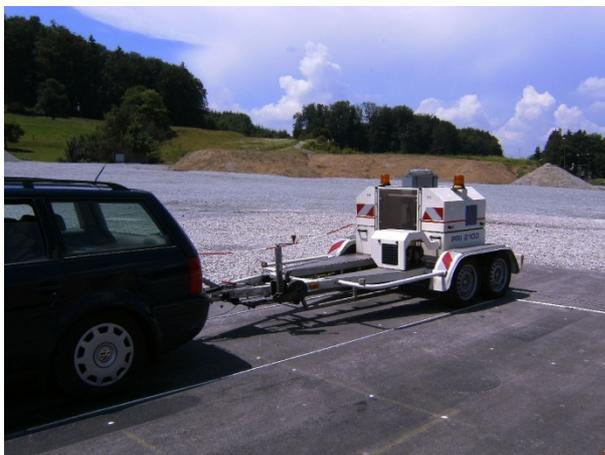
Figure 9: Falling weight deflectometer (FWD).
