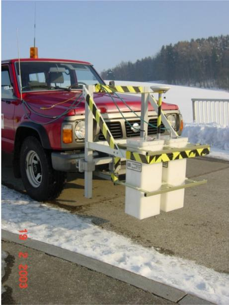
Figure 31: EMPA's mobile acquisition system for pavements and bridge decks.
