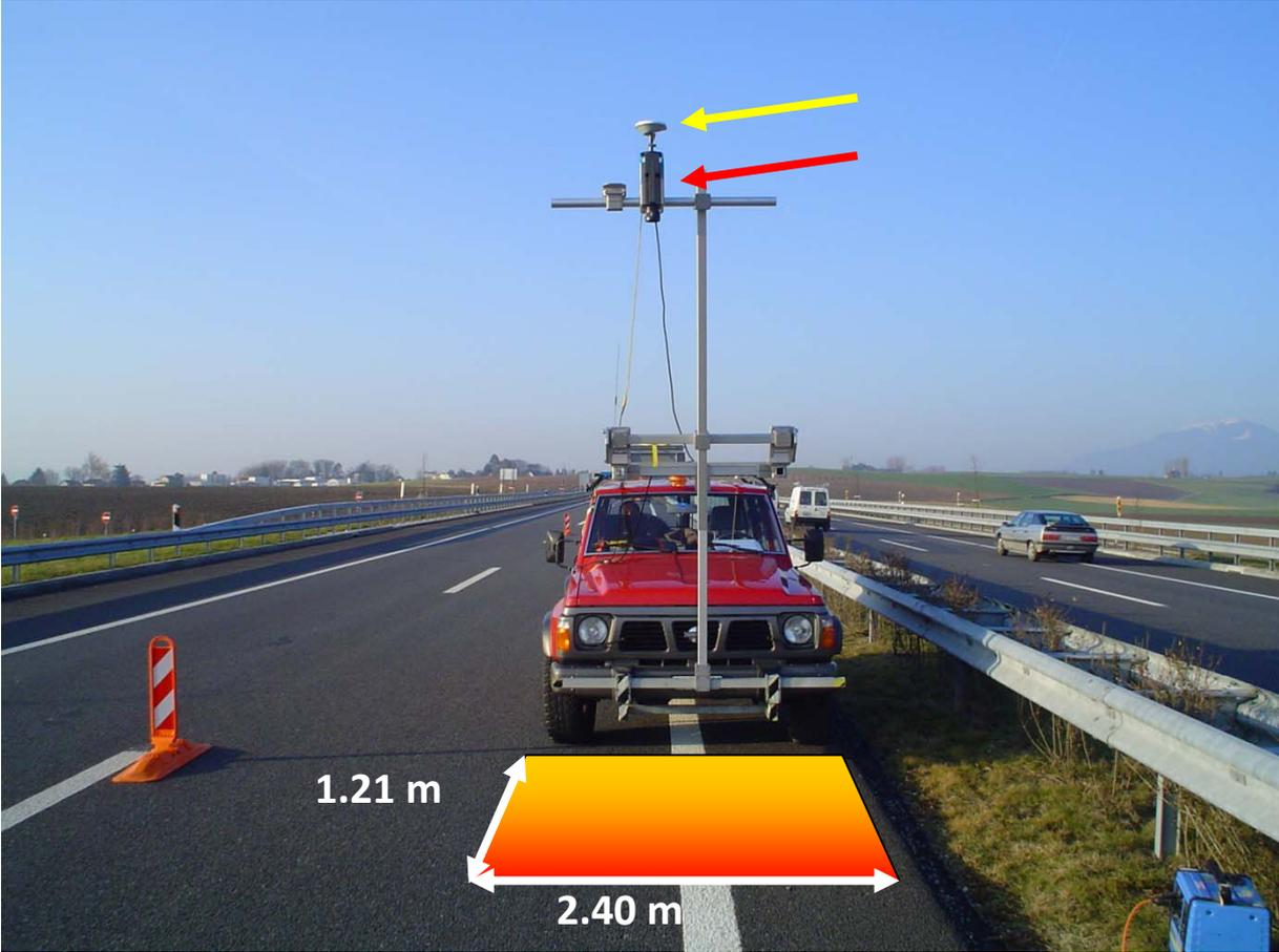
Figure 13: EMPA's mobile IR-system.
