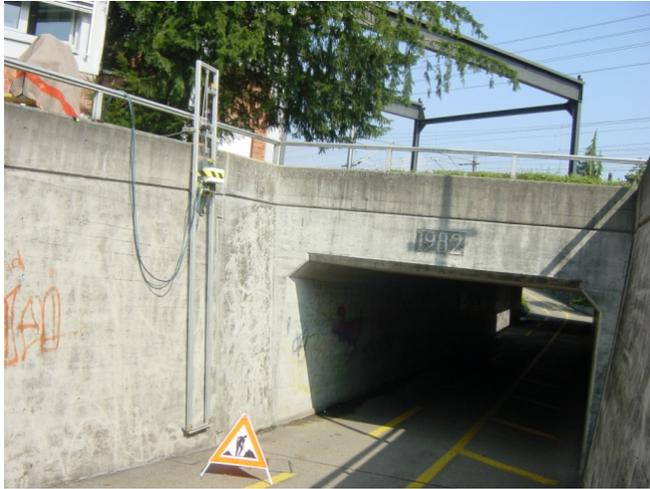
Figure 87: Retaining wall with acquisition apparatus.
