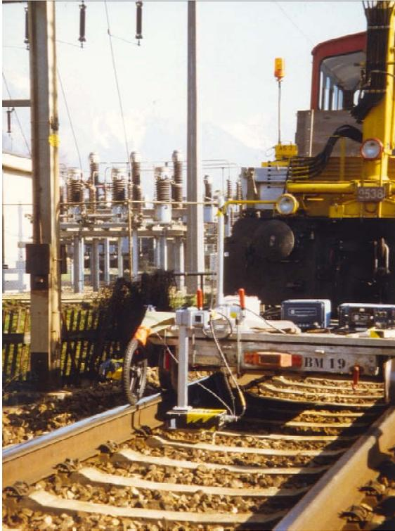
Figure 125: Set-up for mobile data acquisition on railway tracks.
