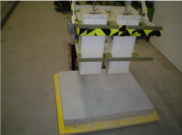
**Figure 58: Antennas positioned above specimen during data acquisition.**
