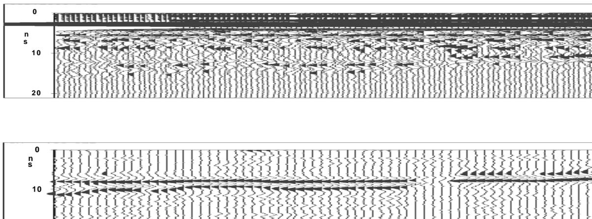
Figure 127: Comparison between data set before (top) and after processing (bottom), site 2, profile length 40 m.
