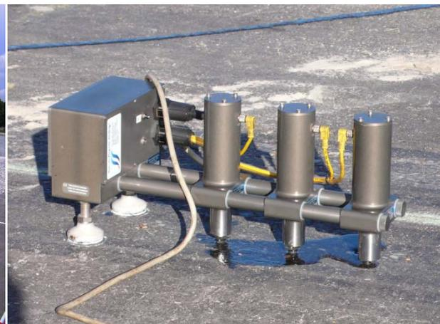
Figure 10: Portable seismic pavement analyzer (PSPA).
