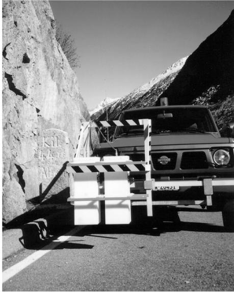
**Figure 140: EMPA's mobile GPR system.**
