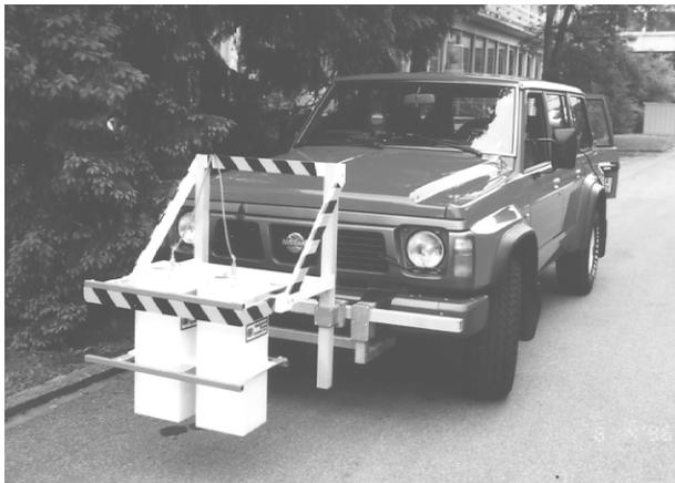
**Figure 111: Vehicle mounted horn antennas**
