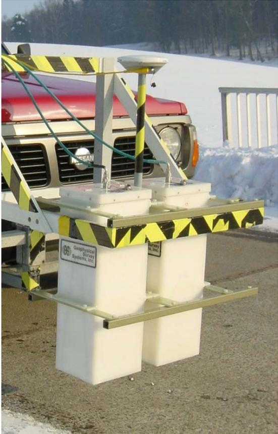
Figure 23: The GPS antenna centered above the horn antennas.
