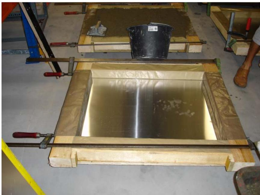
**Figure 57: Mould for the production of the specimens.**
