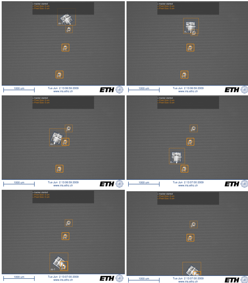
Figure 8.3: Pushing disks using a MagMite. The disk and the MagMite have the same color information but can be distinguished even when they are joined using prior information on each object's position. The arrow on the microrobot indicates its orientation. Similarly, the orange circle and the white dot denote the position of the disk. The squares show the region of interest where the tracker is updated for each object.
