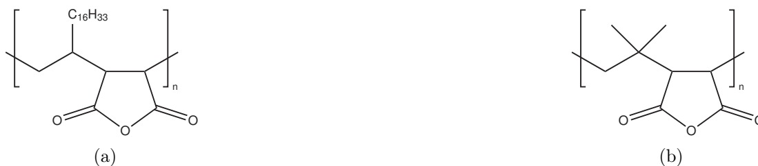
Figure 2.2: Schematic drawings of both reactive backbone polymers used in this thesis, (a) Poly(maleic anhydride-alt-1-octadecene) and (b) Poly(isobutylene-alt-maleic anhydride)
