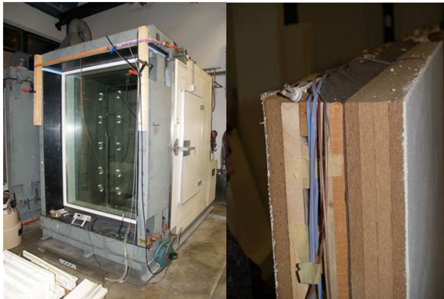
Figure 3-3: Climate chamber (left) and test piece (Wall type A) (right)
