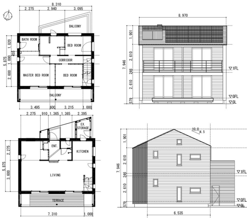
Figure 4-6: Test House (upper left: floor plan of the 1st floor, lower left: floor plan of the ground floor, upper right: south façade, lower right: east façade)
