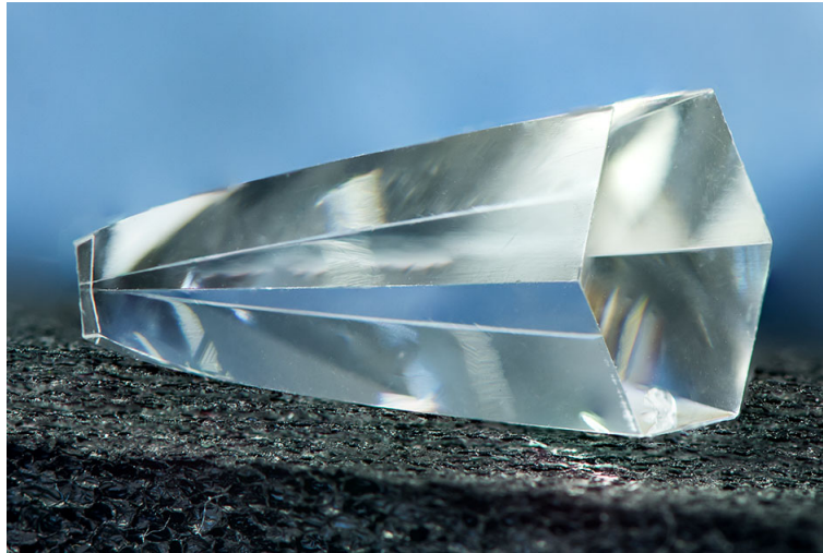
Figure 3.17.: Geometry of the final cones for FACT: the hexagonal entrance area is concentrated by a factor of ten onto the square exit area. Four of the six corners of the entrance area are connected via an edge to the corners of the exit window, whereas the other two edges vanish into opposite sides of the square.
