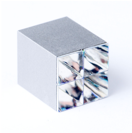
Figure 3.5.: Assembled cone for the prototype module M0: the light is concentrated by reflections on the flat sides of the cone onto the sensitive area of the photosensor. 4 cone-photosensor pairs form one pixel of the module.
