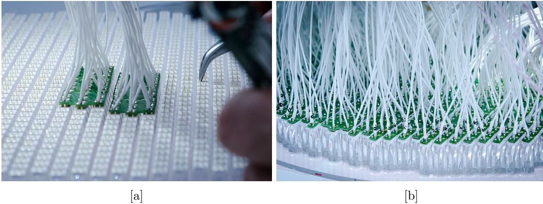
Figure 3.54.: Soldering of the cables to the G-APDs: [a] The G-APDs are soldered to small circuit boards, which are connected to the coaxial signal cables. Each board is for one patch (9 pixels). The 18 pins must be exactly parallel in order to fit the boards. [b] The cables were soldered from the center of the camera towards the outer ring, since the cable density made it difficult to access pixels after their neighbors were connected.
