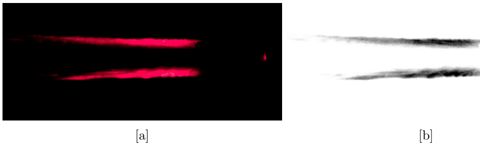
Figure 3.27.: Processing of the reflection images: the original images from the photo camera (left) were converted to grayscale and inverted (right) for the comparison with the simulation.
