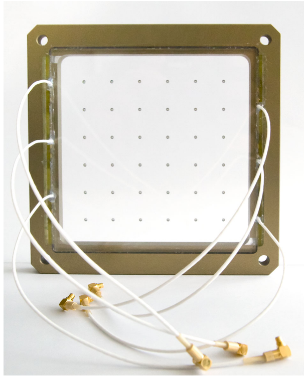
Figure 3.7.: The PMMA front window is equipped with LEDs at the side to provide a reference light pulse. Small holes were drilled into the surface of the window to act as light scattering center. Photo courtesy of Q. Weitzel.
