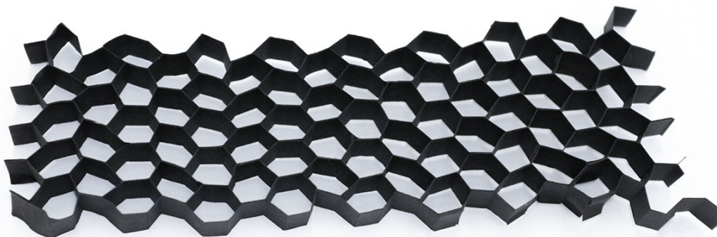
Figure 3.19.: The second grid was a handmade light-weight structure from black paper. Since it is flexible, it would have been easy to place over the final pixel structure. Its main disadvantage was its unknown long-term behavior.
