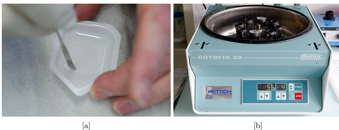
Figure 3.39.: Preparation of the glue: [a] The two components of the glue were weighted and mixed carefully. [b] To get bubbles out of the glue, the syringe was put into a centrifuge at 500 rpm/min for four minutes.
