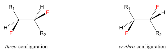
Figure 40. Two general cases of possible vic -difluoroalkyl derivatives: the threo and erythro configurations.
