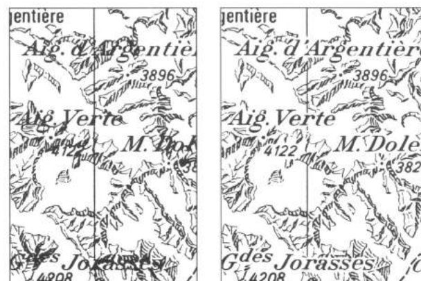
Fig. 2.218 Lettering used in areas with a high symbol density must be carefully integrated ☺️
