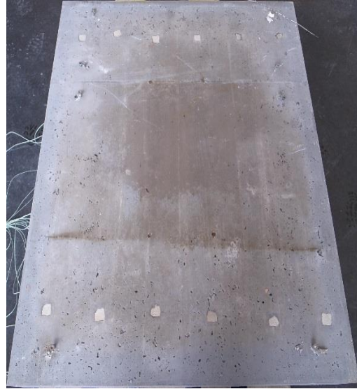
Fig. 2.31 HPC with 18 mm of protective plate after 120 minutes of ISO-fire exposure.
