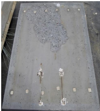
Fig. 5.40 Spalled HPC slab after 14 minutes of ISO fire exposure.
