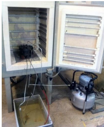
Fig. 3.4 Furnace including permeability testing device.
