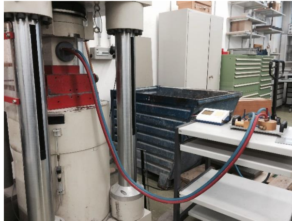
Fig. C.1 Test setup for the permeability measurements under axial compressive stress.
