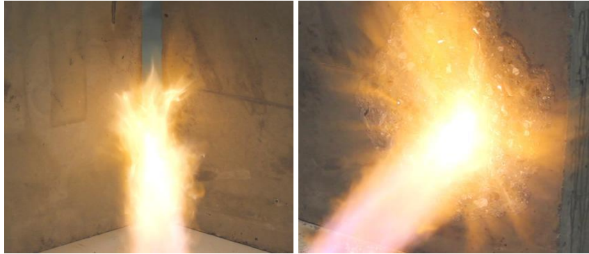
Fig. 2.25 Heating of the corners and center of the specimens (Jansson and Boström 2012).
