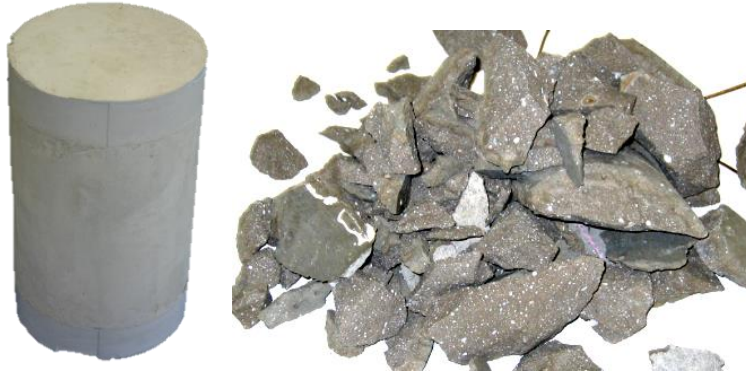
Fig. 2.23 Specimen (cylinder d=150mm, L=300mm) before and after the test with a low heating rate of 0.5 K/min (Klingsch 2013).
