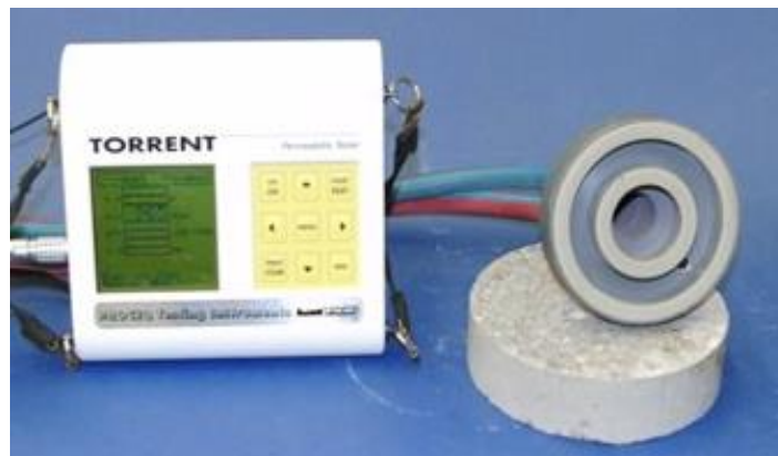
Fig. 3.5 Residual permeability measuring device according to the Torrent method.
