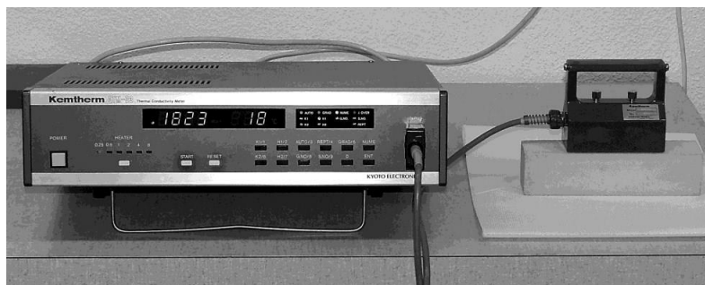
Fig. 5.14 Measurement of initial thermal conductivity.
