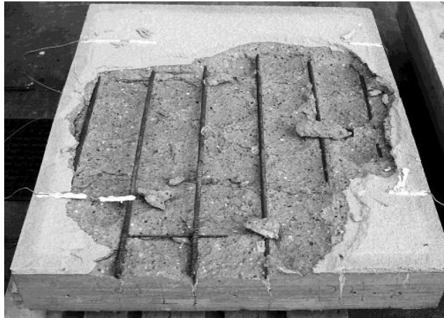
Fig. 5.12 Spalled HPC slab with 10 mm of protective mortar.
