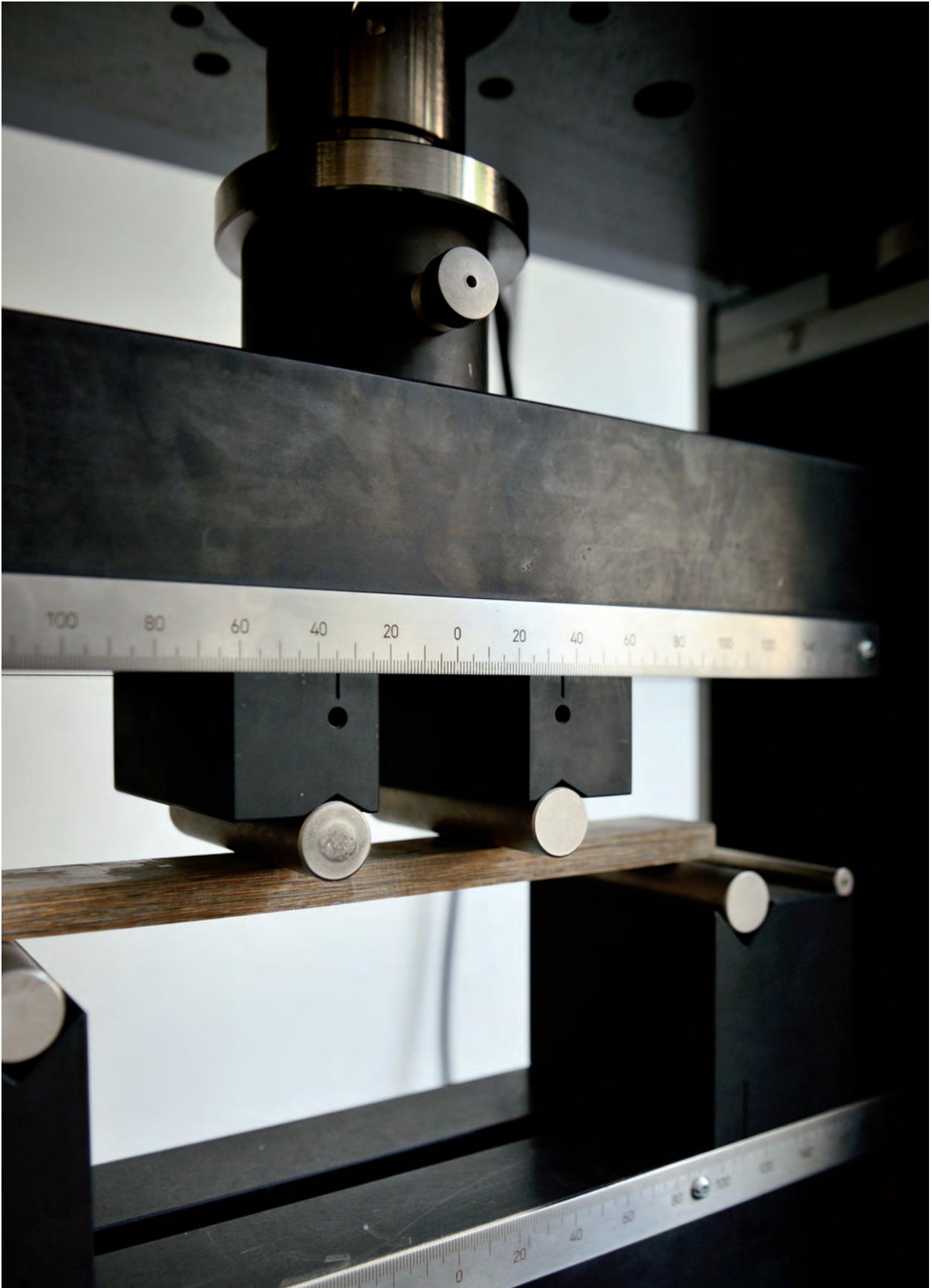
Fig. 01 Bending test at the Advanced Fiber Composite Laboratory in Singapore
