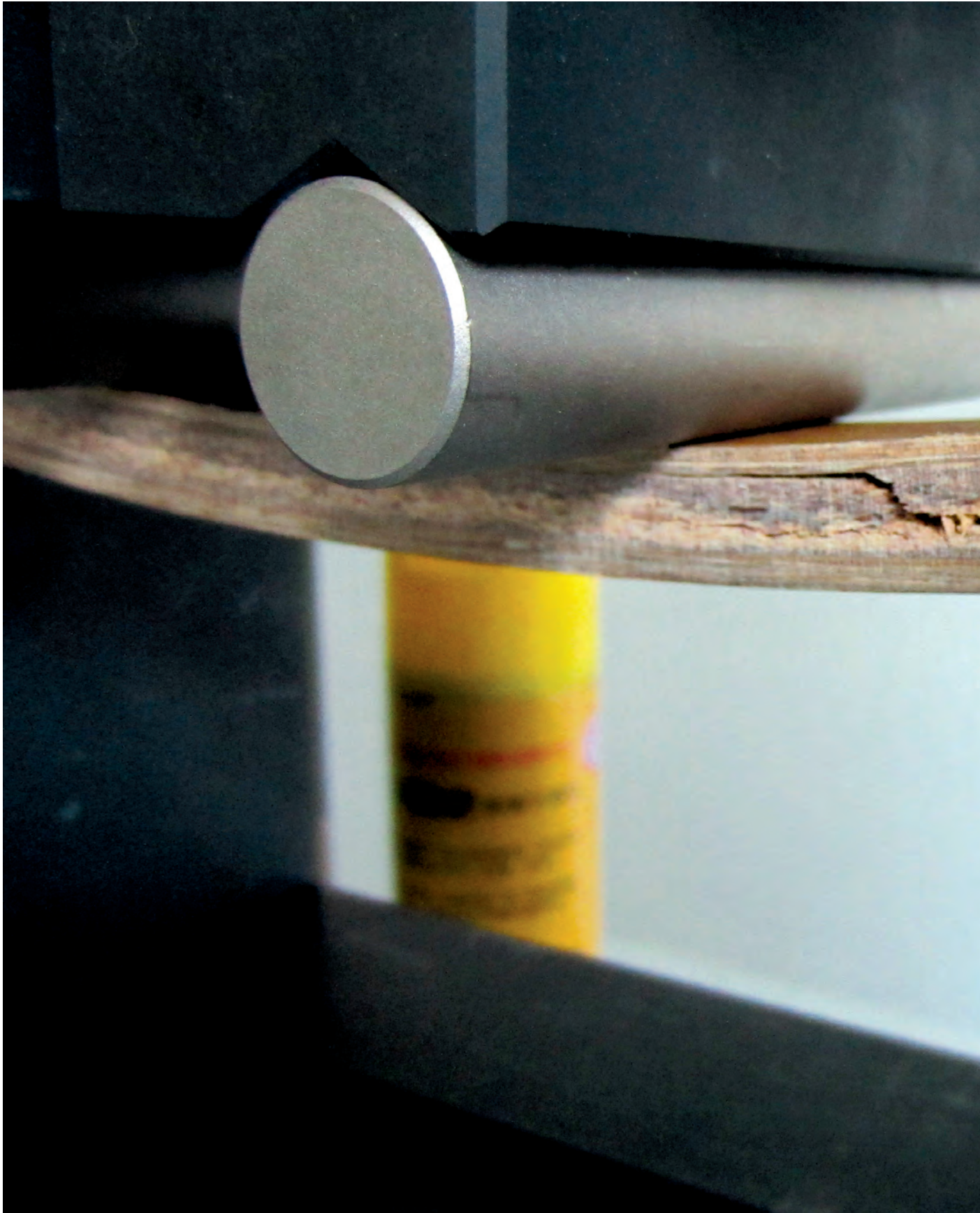
Fig. 03 Shear failure in Bamboo Composite Laminated chipboard
