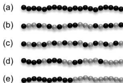
Figure 1-1: Schematic representation of linear polymer microstructures encompassing homo- (a) and copolymers (b–e). Copolymers can be further divided into random (b), alternating (c), gradient (d), or block (e) copolymers.
