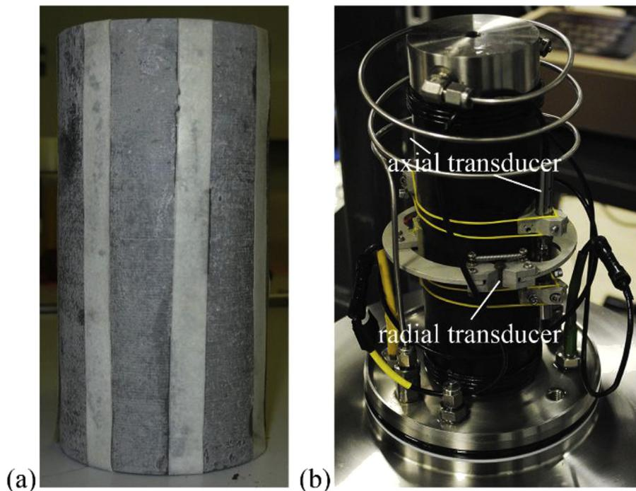
**Fig. 1.** (a) Specimen prepared with filter paper strips at lateral sides; (b) Specimen setup in the triaxial cell with pore pressure line and axial and radial transducers to measure axial and radial displacements locally.
