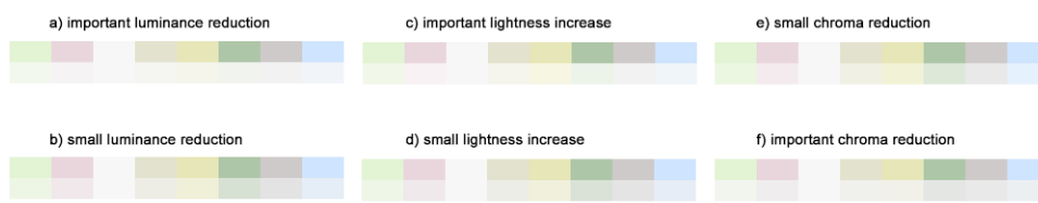
Figure 10. Variation based on the different parameters for a color scheme belonging to a land use layer. For each pair of color scheme lines, the top line of colors is the original color scheme and the bottom line is the modified one.
