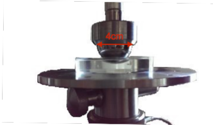
Figure 3.1 | Compression test machine for macroscopic mechanical characterization
