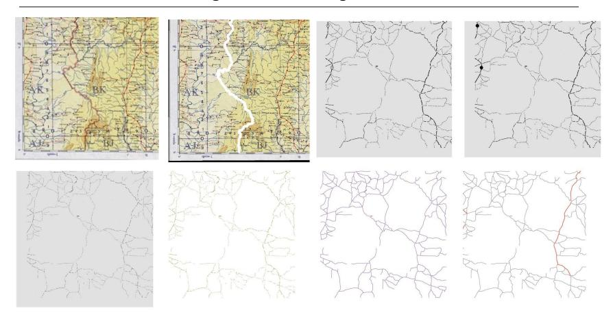
Original – Pre-Treatment – Pixel extraction – Removing circles – Skeletonisation – Vectorisation – Line snapping – Classification
