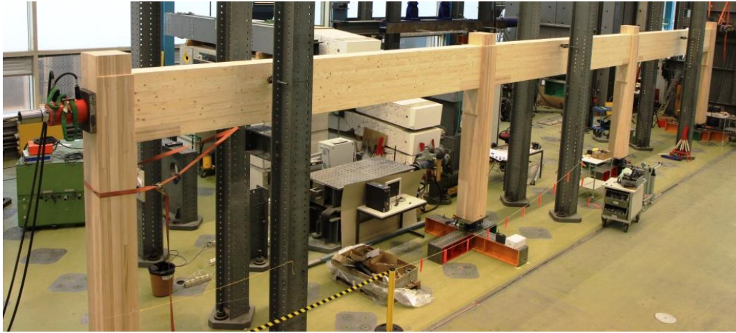
Fig. 1.1: Three-bay post-tensioned frame test setup on the strong floor at the ETH Zurich
