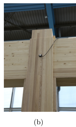
Fig. 2.9: 2.9(a): Accelerometer setup 2.9(b): Picture of a 3-axial MEMS accelerometer attached to a column
