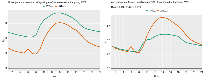
Figure C.10.: Diurnal cycle of hourly air temperature as measured at Kyanjing AWS (KYA) and Langtang AWS (LGT) in 2014 (left) and as measured at LGT and lapsed to LGT from KYA (right). ‘Bias’ and ‘NSE’ show the bias of the lapsed values from the measured data and the Nash-Sutcliffe efficiency (Nash and Sutcliffe, 1970), respectively, both based on hourly temperature data.
