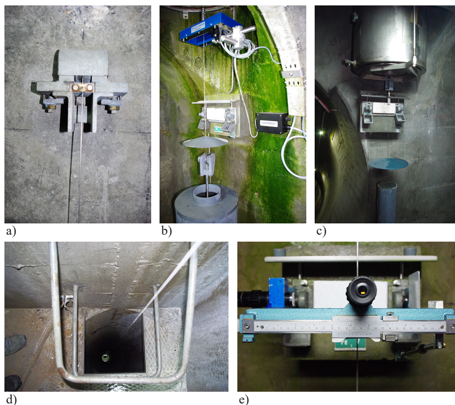
Fig. 2.11 Equipment to measure displacements by pendulum: a) fixed pendulum at the top; b) direct pendulum with electronic reading at the top; c) inverted pendulum; d) vertical shaft with pendulum wire; e) device for manual pendulum reading (photos: M. Bühlmann).
