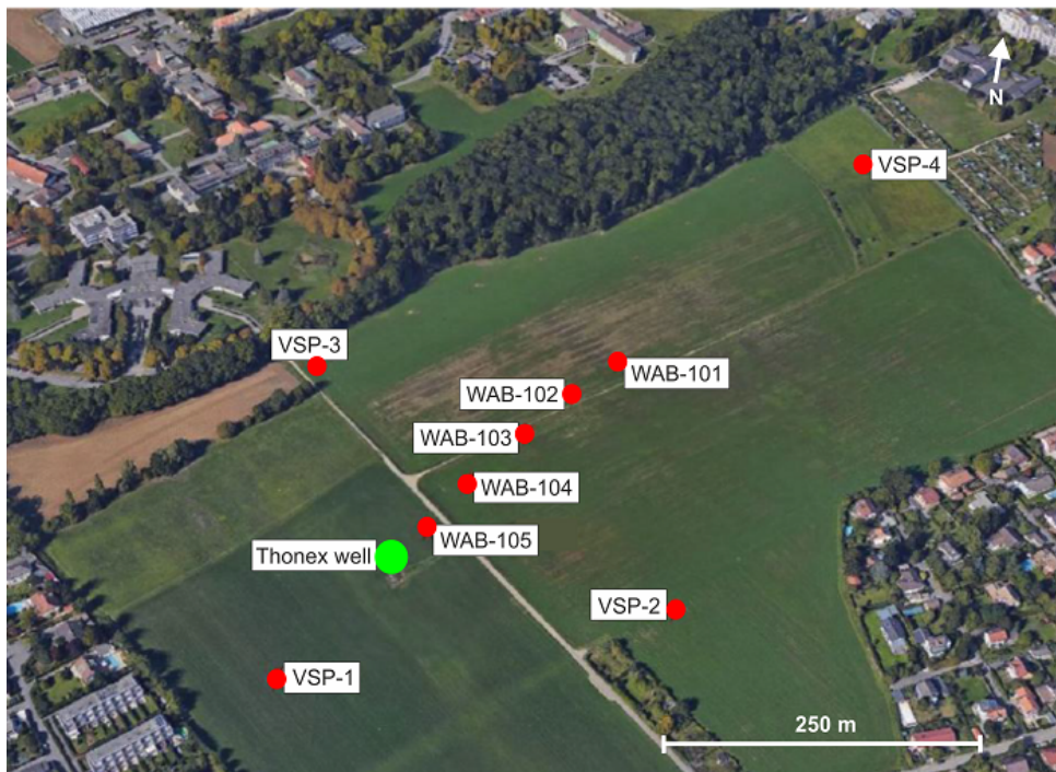
Figure 4.1: Survey layout of the VSP experiment in Thonex. The offset VSP's are marked with VSP-1-4 and the walk-above source positions with WAB-101-105 (modified after Corubolo et al. (2017)).
