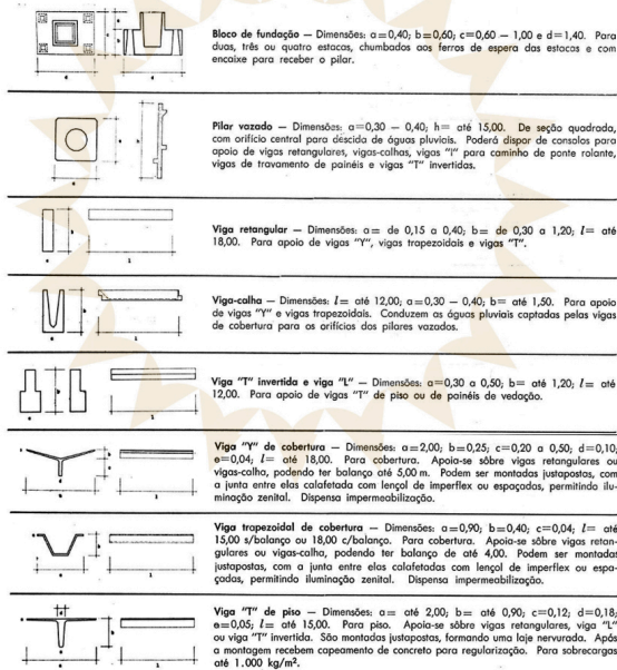
Fig. 2.52 Cinasa system catalog. Prefabricated elements in reinforced concrete. Acrópole , no. 380 (1970): 41-42
