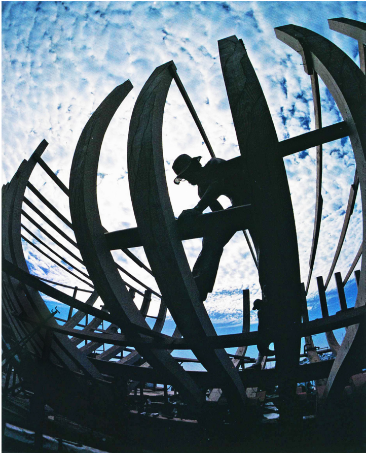
Fig. 2.105 Shipbuilding. Ribbed structure ( Cavername ). Joseph Gribbins, Woodenboats: vom Ruderboot zur Luxusyacht (Stuttgart: Pietsch, 2004), 41
