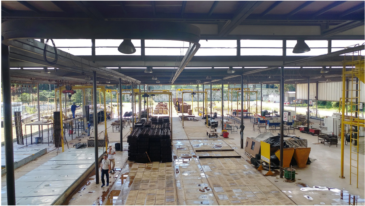
Fig. 3.72 Overview of the argamassa armada workshop at the CTRS showing the four production lines, the sliding gantries and the electric hoists. Photograph by Akemi Tahara, 2017. Courtesy of José Fernando Minho
