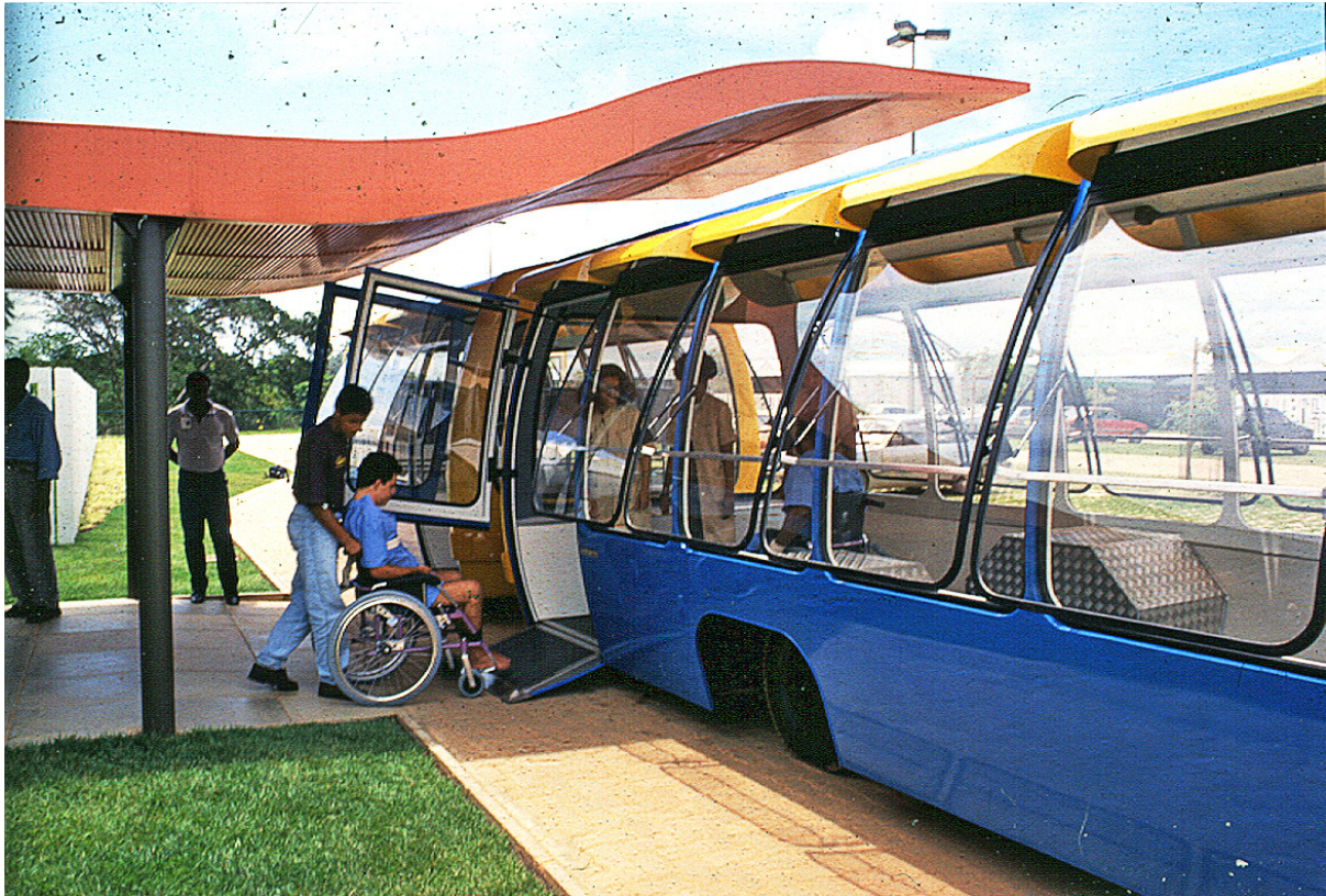
Fig. 2.119 Entrance marquee of the Sarah Hospital in Salvador, Bahia. The curvature of the element allows the shuttle bus (designed by Lelé's team) to get closer to the entrance, therefore making it easier for the patient to board. Arquivo JFL, Salvador
