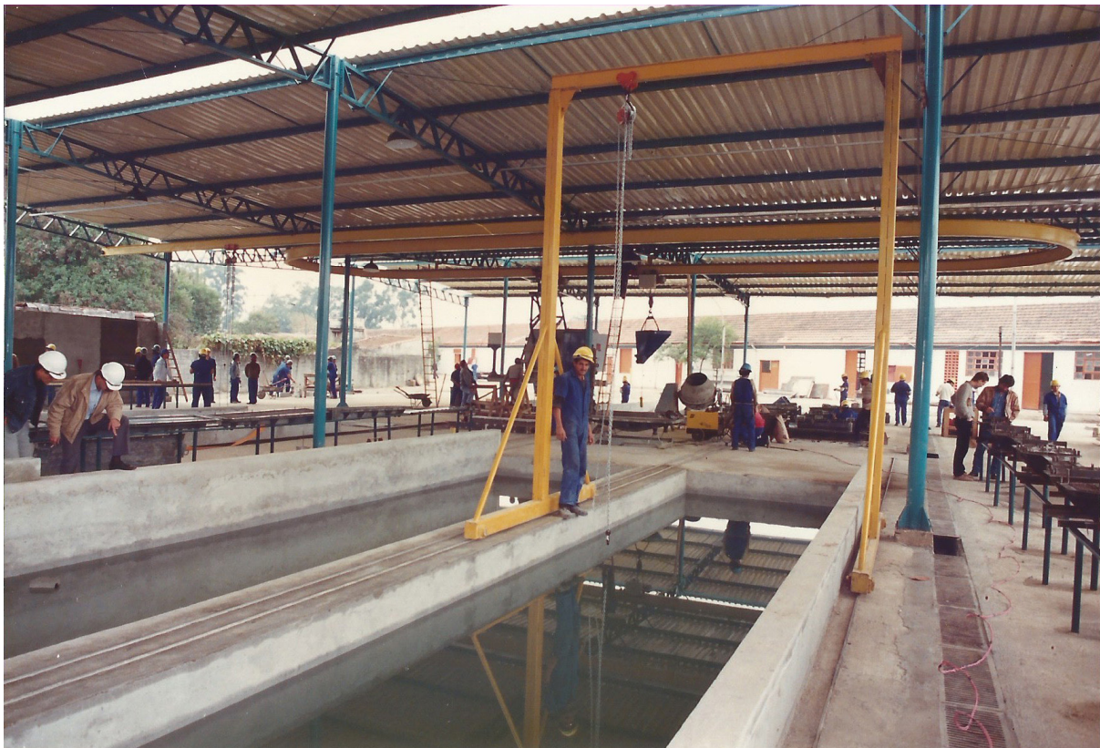
Fig. 3.58 CEDEC factory in São Paulo. Production area. Curing tanks with water before their adaptation to vapour chambers. Arquivo Paulo Eduardo Fonseca de Campos, São Paulo
