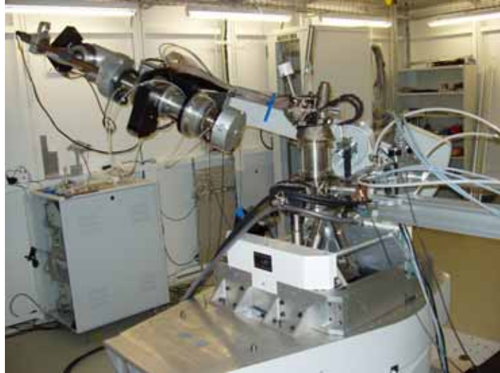
Fig. 1.1 Portable UHV chamber mounted in the horizontal set-up on the (2+3) surface diffractometer at the Materials Science Beamline at SLS.
