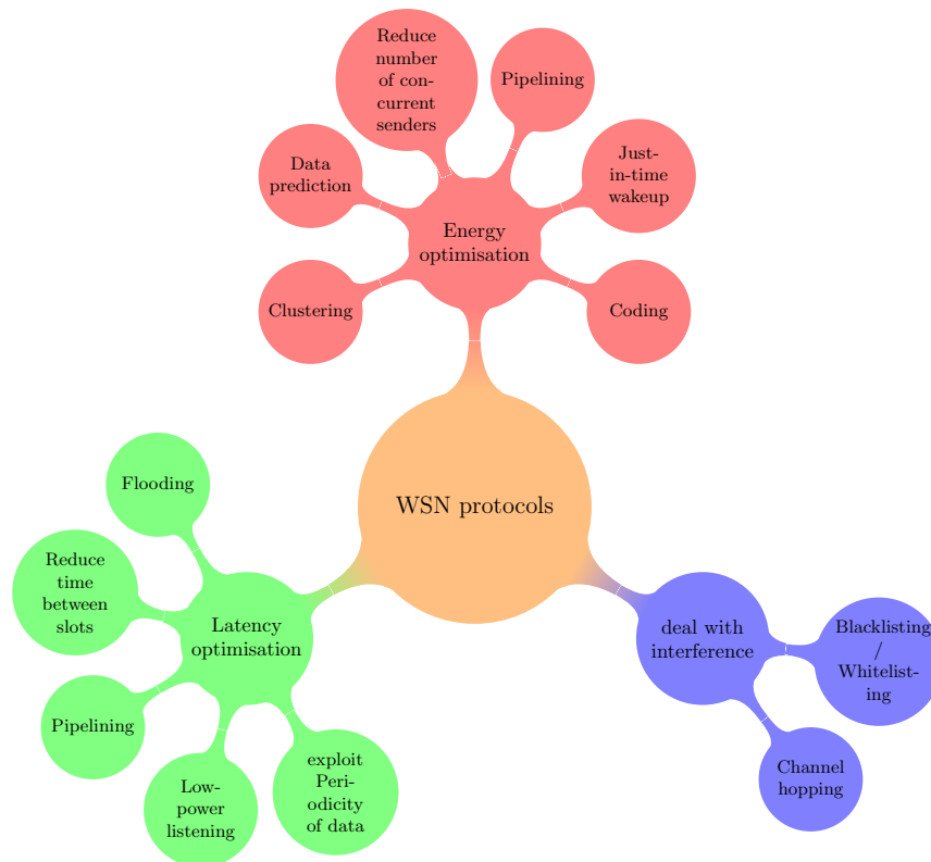
Figure 2.2: This is an overview of ways to improve certain protocol performance metrics.
