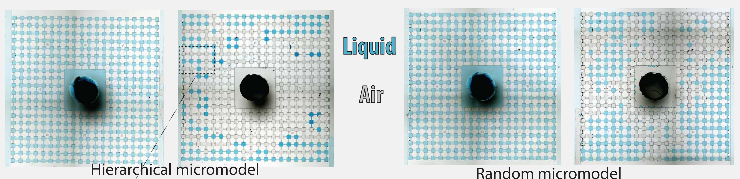
Fig. 6. Aqueous distribution in hierarchical and random micromodels before and after fragmentation imposed by air entry through the central square. Close-up shows fragmentation paths (red arrows) driven by channel size
