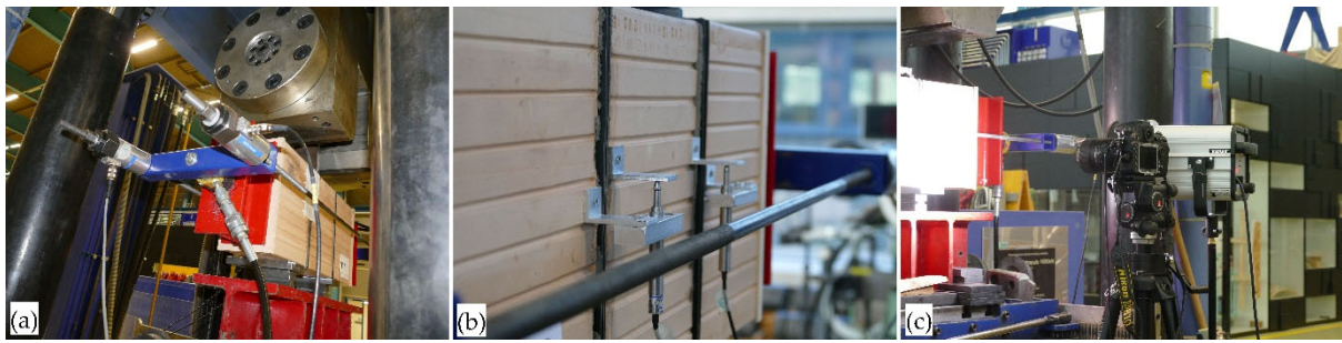
Fig. 6. Measuring devices: a) loading cells; b) LVDTs; c) DIC system
