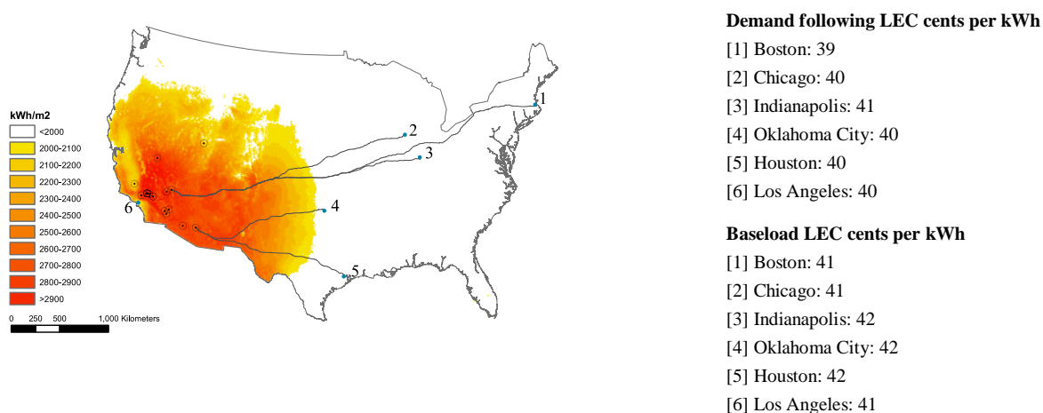
Figure 3 Levelized electricity cost at point of demand for the United States when supplied by a CSP fleet at existing/planned sites.
