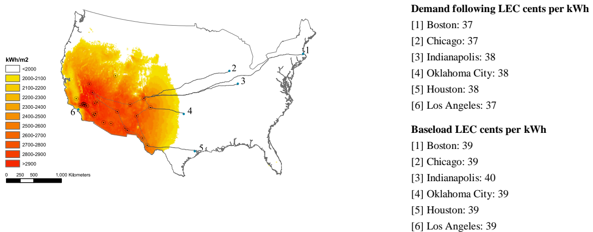
Figure 4 Levelized electricity cost at point of demand for the United States when supplied by a CSP fleet at all suitable sites
