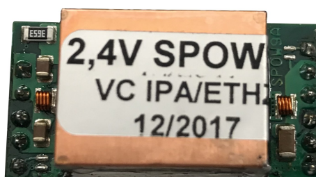
Figure 2. A picture of the developed device, the main shield as well as the two filters on the in- and output are visible.
