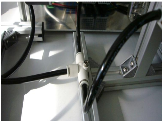
Figure A 25. Connection of mechanical pressure station 2 to the bottle for wash solvents.
