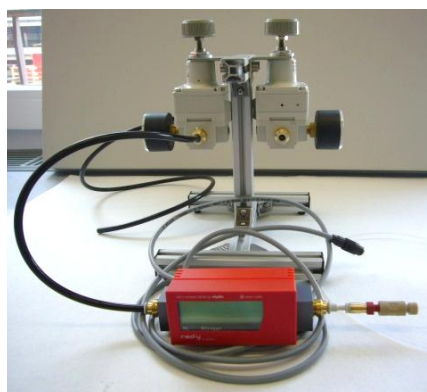
Figure A 11. Gas flow meter connected to the main gas supply.
