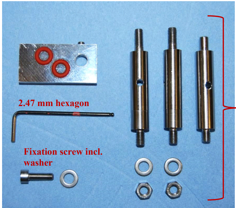
Figure A 72. Tools for fixing the sampler at the ESI source basis plate.
