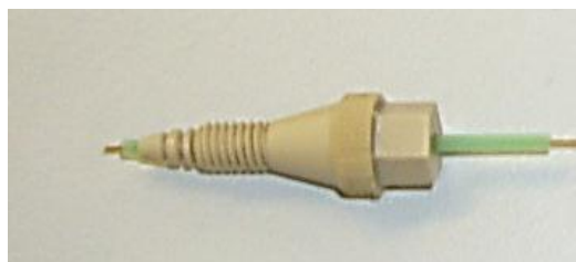
Figure A 41. A hexagon-headed PEEK finger tight, double grip ferrule and a green sleeve.
