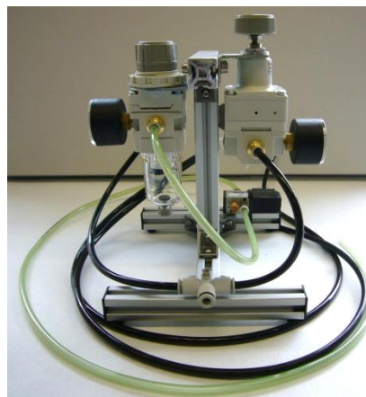
Figure A 17. AW20-F02BM pressure regulator (step 3).
