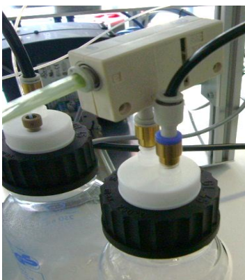
Figure A 27. Connection of mechanical station 1 to the inlet of the Bronkhorst IQ flow gas regulator.
