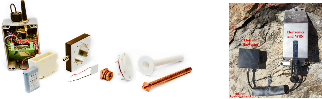
Figure 8. Left: exploded view of the system components of the harvesting system consisting of the thermal harvester, TEG, rectification circuitry, and the wireless sensor node (WSN). Right: the system deployed in the rock wall for the long-term case study (photograph of the SE position 29).
