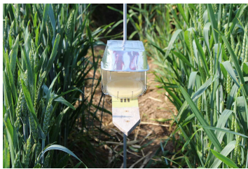
Fig. II.2. Spore traps with Fusarium selective medium placed between two adjacent wheat varieties and adjusted to the same height as the flowering heads.
