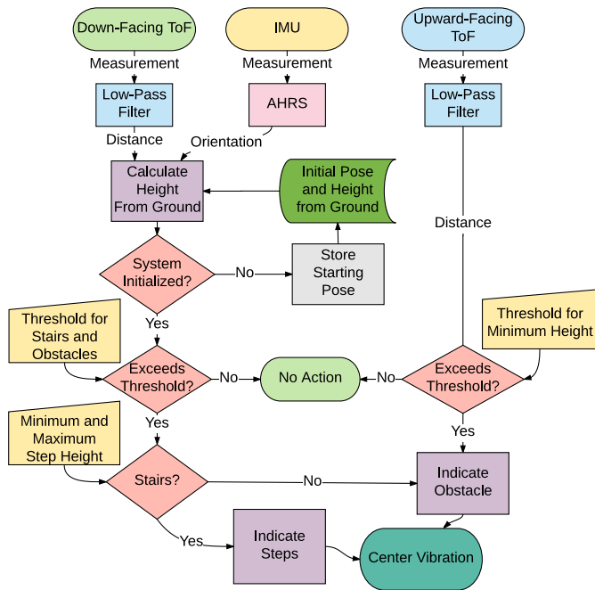
Fig. 6. Low- and High-Obstacle Detection and Indication: The flow chart outlines the steps of detection, processing, and feedback generation in the case of low or high obstacles in front of the user.
