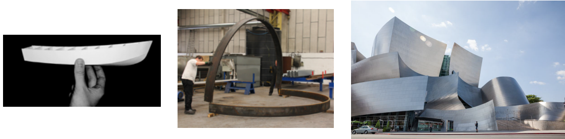
Figure 1.4: Developable surfaces are easy to build, but hard to design. Developable surfaces are prominent in the manufacturing industry and in architecture. Left - ship hull design by [Pérez and Suárez 2007], center - bending of metal by Bernshaws, right - Frank Gehry's Walt Disney concert hall (photo by Jon Sullivan).
