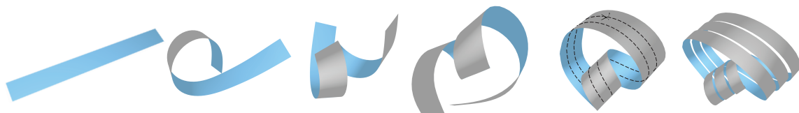
Figure 6.8: Our local isometry model allows us to deform, glue, and cut a surface while maintaining an exact discrete notion of local isometry. In this figure we twist a long strip twice, glue it, and then cut it along two horizontal sections, creating three interleaved knotted surfaces.
