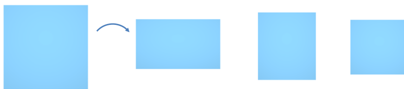
Figure 1.5: Intrinsic deformations of a developable surface. While one might prefer to limit stretching when modeling, allowing for stretching a developable surface can in fact be beneficial for editing tasks, since this does not limit the model to a fixed reference isometric sheet, which is often unknown during the design phase. Strictly modeling isometries in our model is tackled in Chapter 6 and modeled in Chapter 7.
