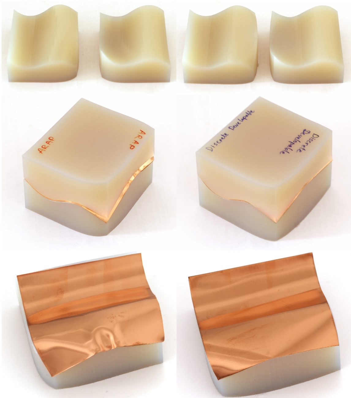
Figure 3.13: Validation by fabrication. We 3D-printed a “sandwich” (top row) whose inner cut surface is the result of deforming a flat square using ARAP (left column) and our editing system for discrete developable surfaces (right column) using the same (soft) positional constraints. We cut two squares out of a thin copper sheet with the dimensions of the initial model before deformation, and we sandwiched these squares in the fabricated pieces (second row). Not surprisingly, since the ARAP result is not developable, the sheet wrinkles and buckles (bottom left), while our result exhibits pure bending (bottom right). Note that our result is smooth everywhere except at the boundary, where a cone-like kink is created in the digital model to remedy the doubly curved ARAP surface.
