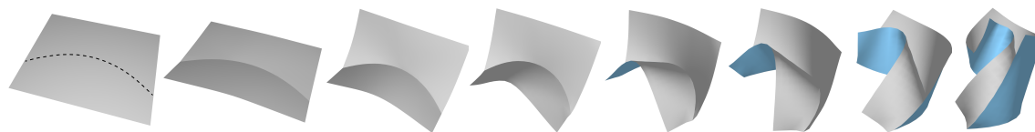
Figure 7.4: Homotopy based optimization for curved folding modeling. A discretization of a curve-constraining flow on curved crease surfaces, composed of two DOG patches connected by boundary constraints. This folding and bending flow is smooth, when viewed on the patches separately. connected along used in the above animation.
