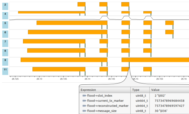
Figure 6: With the debug service, a breakpoint is set on the first TxDone interrupt on node 9. This allows to extract the values of the internal variables at that point in time.
