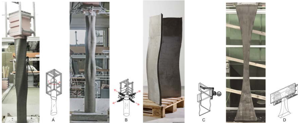
Figure 2.14: Different formwork typologies used in Smart Dynamic Casting early stage: A) Local deformation rigid formwork that can be configured with different shapes, such as ellipse, circle, square or star shape; B) Local deformation flexible formwork where shaping actuators are only at the exit of the formwork; C) Local deformation formwork for thin folded structures, and D) global deformation formwork for significant cross section change. Source: [44]
