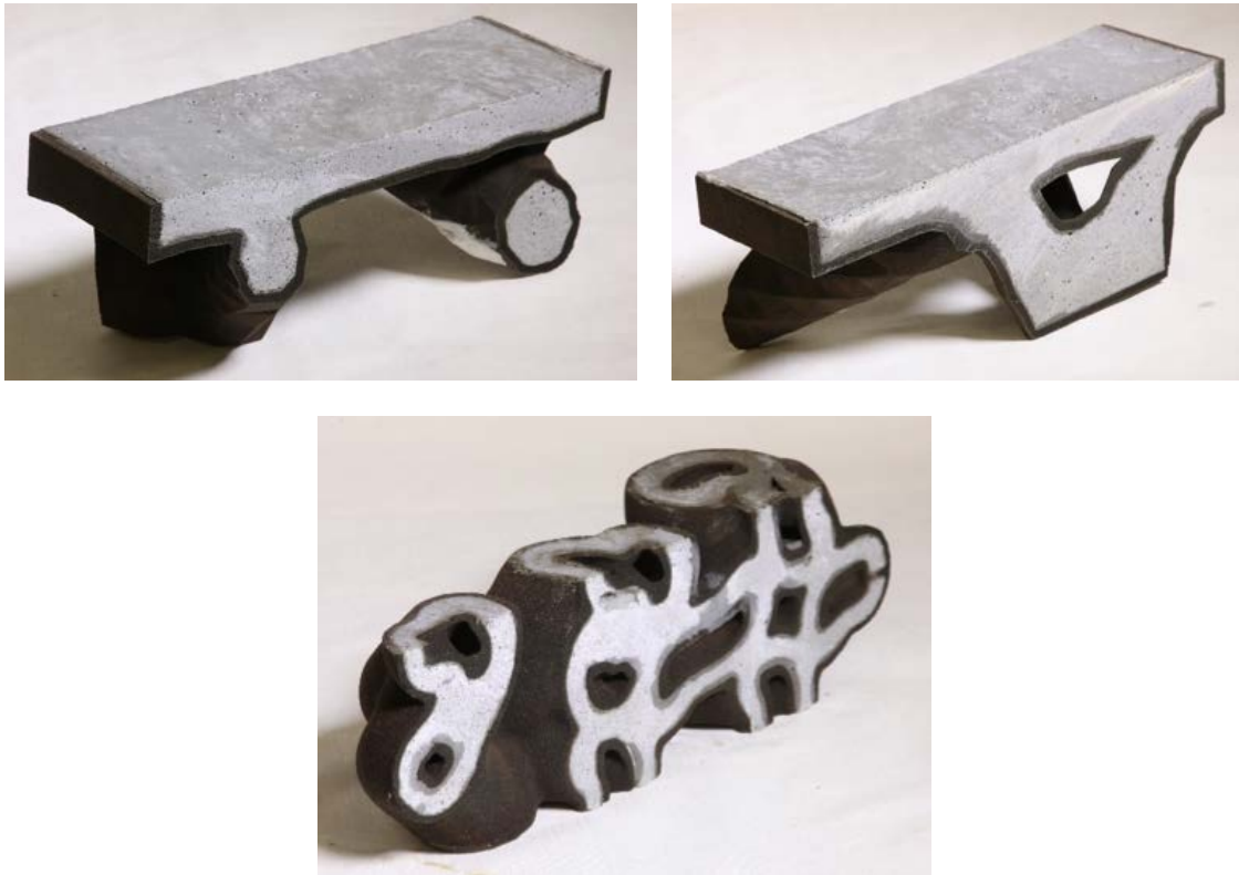
Figure 4.8: Infill testing prototypes, final slab corner (top); abstract cavity (bottom).
