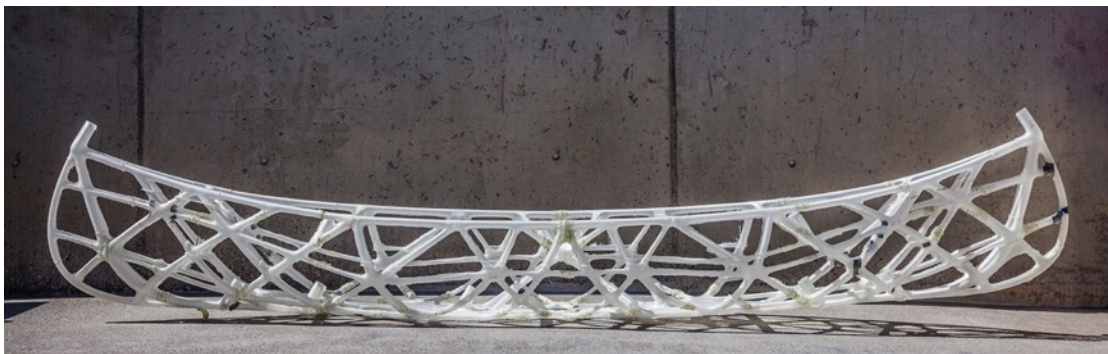
Figure 5.14: The 84 3D printed pieces assembled and ready for casting. (dbt, PCBM, ETH Zürich, 2017)
