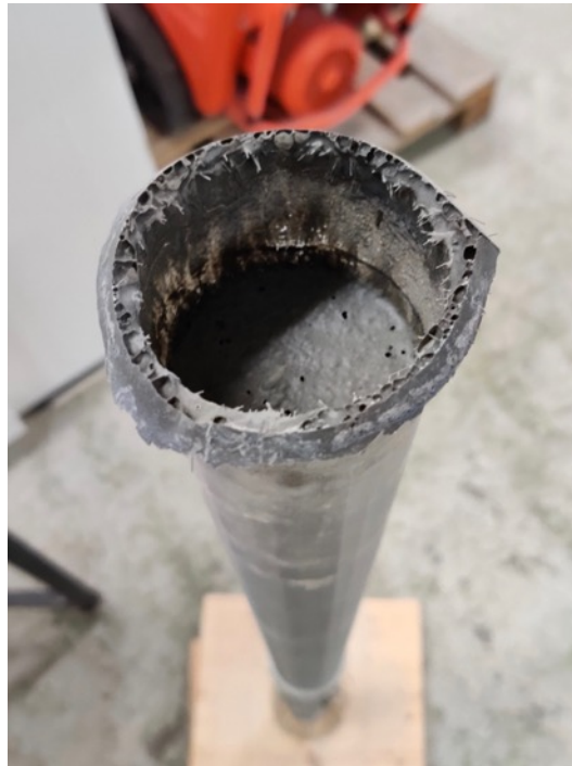
Figure 5.24: Recess of HPFRC on the top of the tube element.
