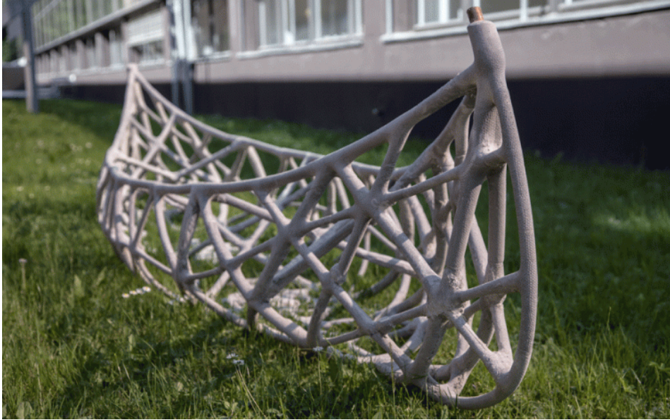
Figure 1.3: Skeletal structure of the concrete canoe. (Photo: dbt, ETH Zürich)
