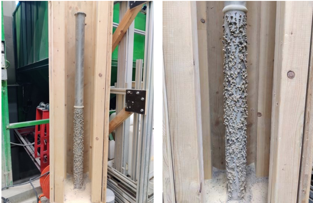
Figure 5.22: Tube element after casting and hardening of the HPFRC and removing of the counter pressure casting sand (both tubes casted with counter-pressure casting were presenting the same kind and pattern of damage). Left: Overview. Right: Lower half.
