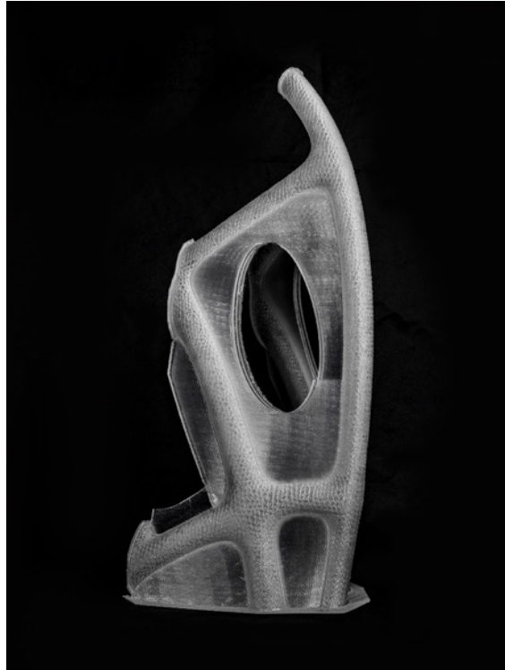
Figure 5.11: A 700-mm tall sample 3D printed part of the skeleTHon formwork. In order to prevent quality issues for taller parts, a membrane-like auxiliary support structure is introduced. (dbt, ETH Zürich, 2017)
