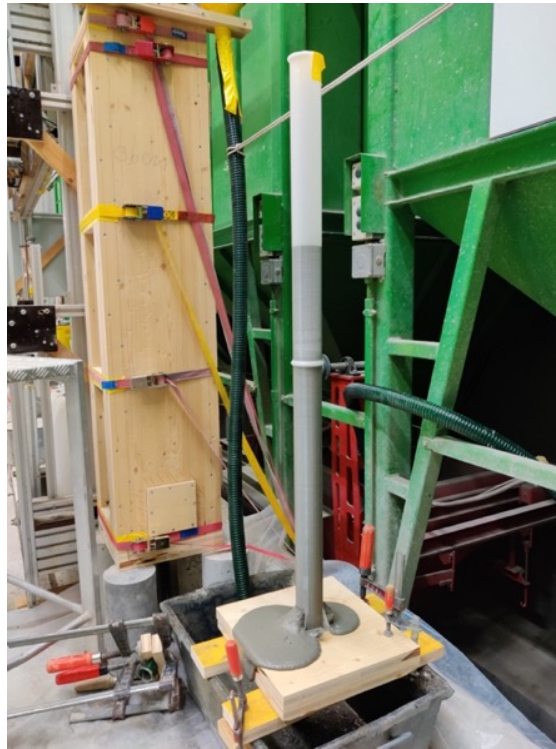
Figure 5.28: Formwork without counter-pressure casting after failure while HPFRC is leaking out. The maximum height the concrete reached in the formwork was 84 cm.
