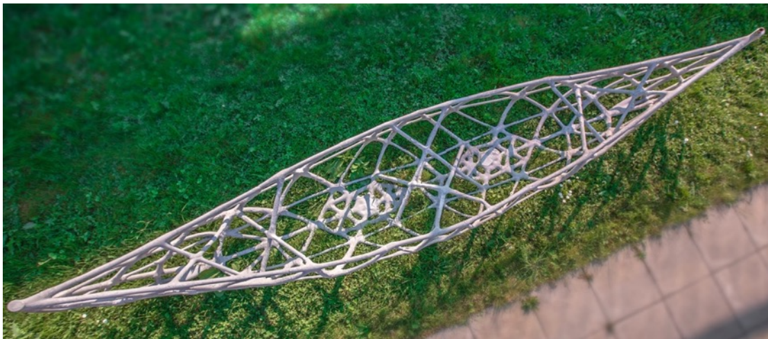
Figure 5.3: The complex concrete “skeleton” that provides the structural integrity for the canoe. (dbt, PCBM, ETH Zürich, 2017)
