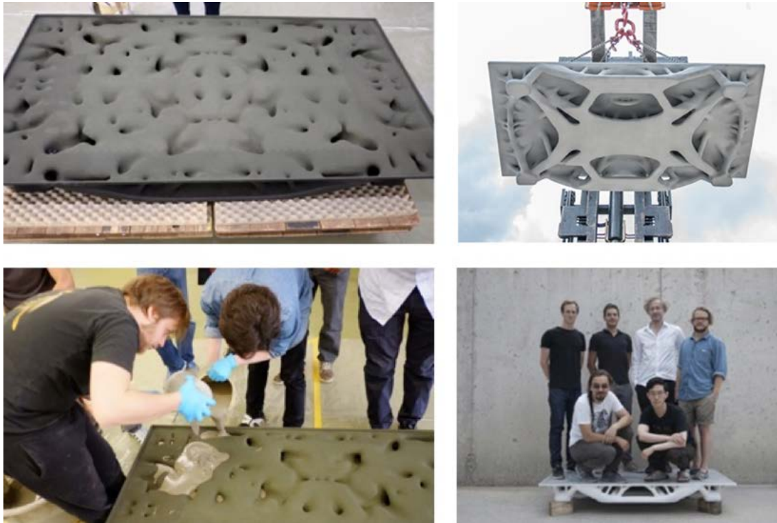
Figure 4.11: Top view of element, pre-infill (top left); Bottom view of element, post-infill (top right); Infill process (bottom left); Final element after casting (bottom right).
