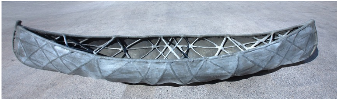
Figure 5.1: skelETHon , the four-metre-long canoe made entirely out of concrete. (dbt, PCBM, ETH Zürich, 2017)
