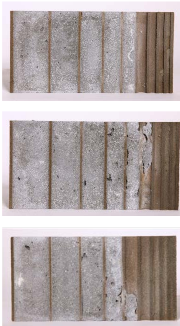
Figure 4.6: Straight tubes with varying diameters (from left to right: diameters of 50, 40, 30, 25, 20, 15, 10, 7.5 and 5mm), 6x0.15mm fibres (top); 10x0.16mm fibres (middle); 13x0.16mm fibres (bottom).
