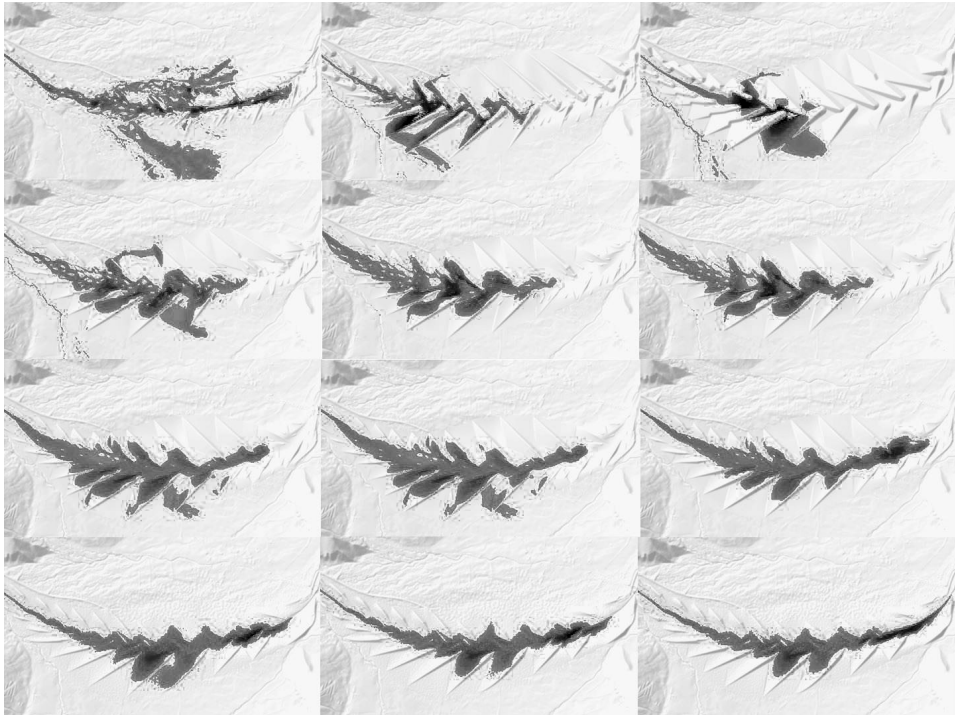
Figure 5.36: Twelve simulations over the course of the whole design process. The first topographic design clearly failed, and was continuously adapted using input from the simulations to come to a valid landscape structure. By students Caspar Trueb and Lorin Wiedemeier.
