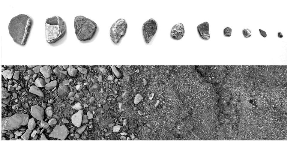
Figure 5.18: Selection of gravel found on the banks of the Bondasca River. The experiments took sand, gravel and boulders into account for the material build-up. By Students Elizabeth Levy and Stanislaw Modrzyk.
