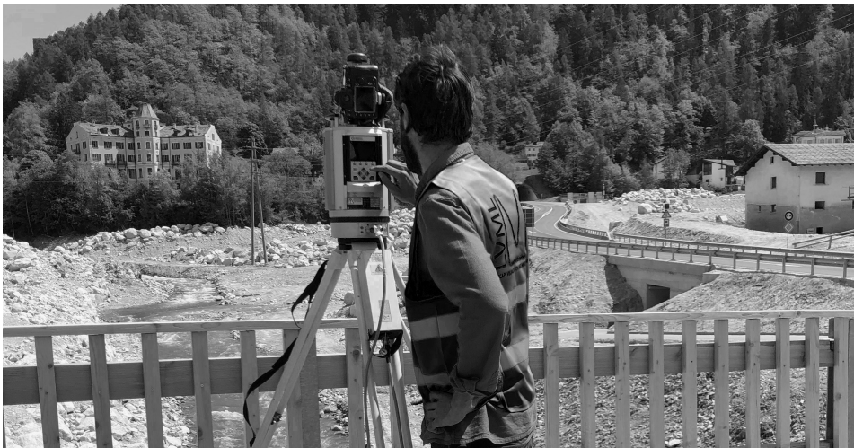
Figure 3.1: Acquisition of a point cloud in Bondo, Grisons using the terrestrial laser scanner Riegl VZ-1000. Photo by Fujan Fahmi.
