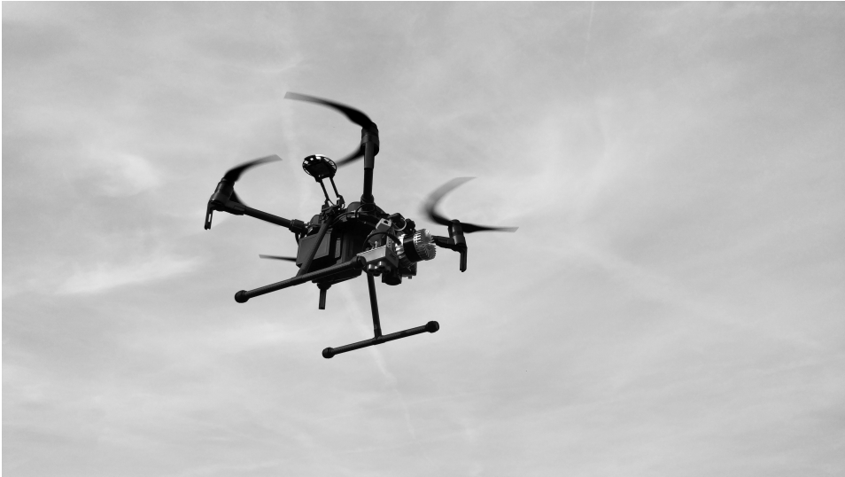
Figure 3.4: Lidar UAV in flight. Implementation of the aerial laser scanner with the lidar system mounted on the front.
