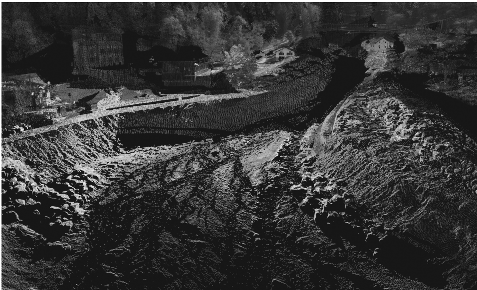
Figure 3.2: Full colour three dimensional point cloud from the terrestrial laser scan of the detention basin for the debris flows in Bondo, Grison.
