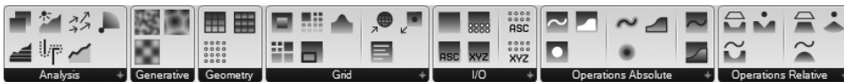
Figure 3.14: The toolbar of Docofossor within Grasshopper where the components are organised in seven categories; I/O., Analysis, Grid, Generative, Absolute Operations, Relative Operations, and Geometry.
