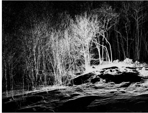
Figure 2.13: Point cloud from a terrestrial laser scan of the forest in Sigrino, Tessin, before the material of the Ceneri Base Tunnel was deposited on this site, from Girot et al. [49].
