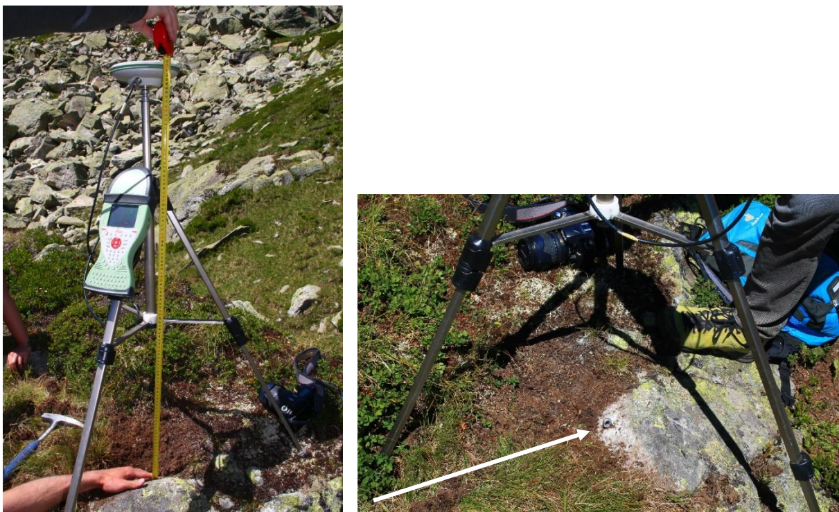
S 3: Measurement of GNSS data in CdV, left image shows tripod with GNSS antenna and the execution of the antenna elevation measurement, right image shows the rock bolt (white arrow) which is used as marker for the respective GNSS point and above which the antenna is placed.
