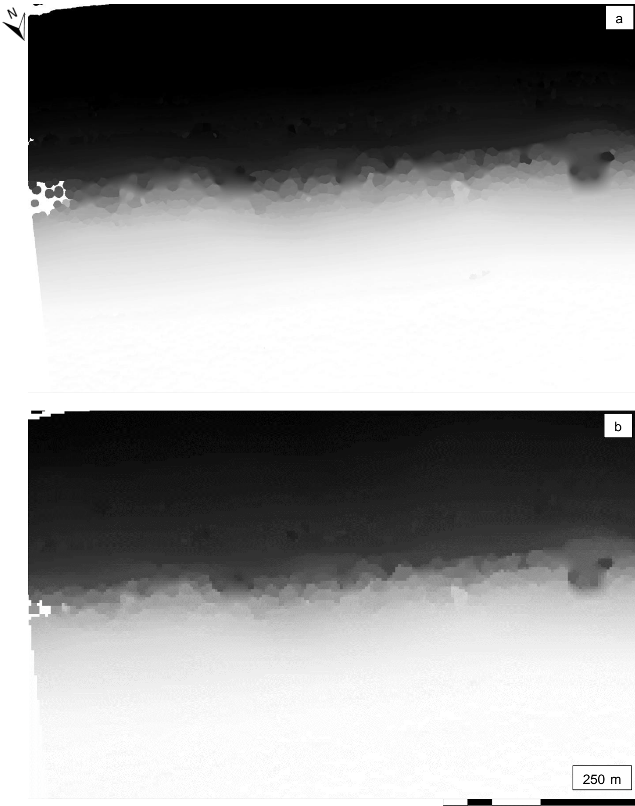
S 16: Qualitative comparison of DEM meshing grid, a) with 10 m resolution, b) with 40 m resolution. a) appears much smoother, but requires significant application of hole filling algorithms, which might lead to severe orthorectification errors. b) appears coarse, but returns much fewer holes and could be preferable for orthorectification. For this work, a 10 m grid was selected, to benefit from the better spatial resolution; potential drawbacks were avoided by a frequent and strict quality control procedure (raw data from HiRISE, n.d.).
