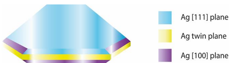
Scheme 2.3 a) Schematic of a silver nanoplate (AgNPI) structure with facets orientation on the nanoplate structure
