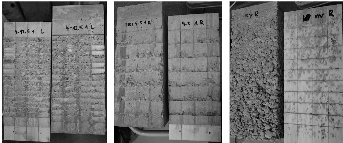
(a) Concrete shear and timber shear (b) Intact notches and timber shear (c) No mechanical connection shear
