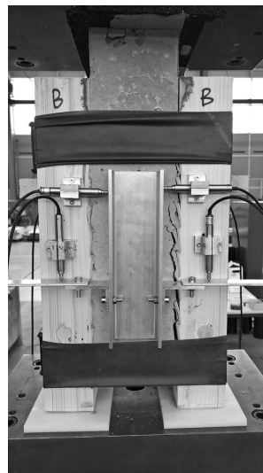
(b) Elastic band installed on a specimen
