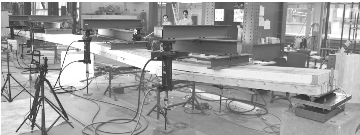
Fig. 6.3: Specimen ZFT2 after failure in one span
