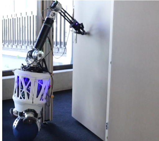
Fig. 1: A ball-balancing manipulator opening a hinged door. The robot is required to maintain its balance and, at the same time, follow a desired end-effector trajectory while interacting with an unknown, external environment.
