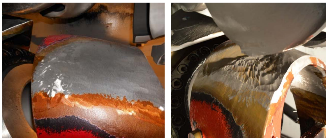
Figure D-20 Deflector of lower nozzle of MG 1 a) in original shape in April 2012 and b) with erosion in August 2012 after the major flood event.
