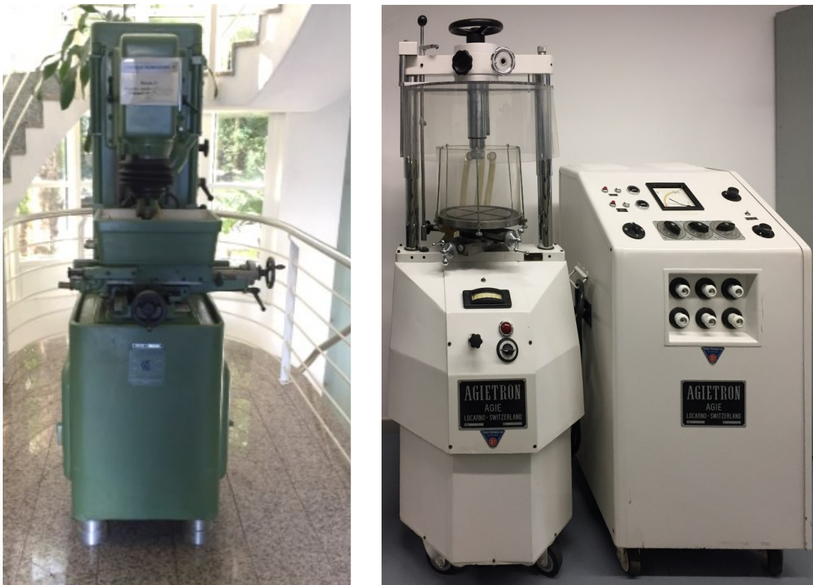
Fig. 1.1: First commercial EDM machines: Left Eleroda (1955, Charmilles); Right Agietron AB (1956, Agie); Photos taken at GFMS research centre, Losone 2019
