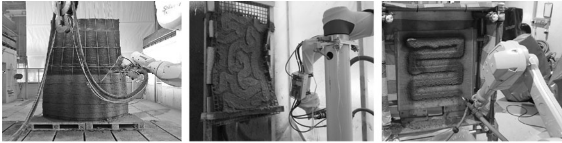
FIG. 2. Left: Shotcrete 3D Printing, investigating freeform concrete elements with high surface qualities, Hack and Kloft. 9 Middle: Robotic AeroCrete, a novel robotic spraying technology for slender, bespoke concrete elements, Taha et al. 10 Right: S-3DCP research investigating the effect of process parameters on material distribution in a spray-based printing process, Lu et al. 11
