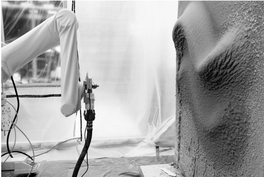
FIG. 10. Preview from a further iteration of the fabrication setup, with an automated plaster spraying tool integrated.
