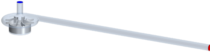
Figure C.1: Overview of the computational fluid domain. Blue: inlet, red: outlet, grey: impeller, translucent: inner wall of housing and extended outflow tubing.
