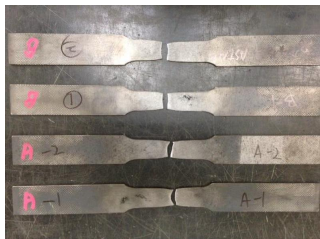
Figure 7.24: (a) Experimental stress-strain curve obtained from coupon tests for the steel grade employed for specimen fabrication, (b) coupon test specimens
