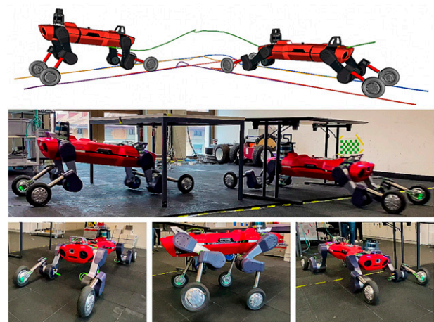
Figure 12. Motion composition of three offline trajectories based on the interactive TO in Section 4.2. The upper visualization shows the torso and end-effector trajectory of the composed trajectory m(t) . Here, the robot executes two ducking motions with a duration of 2 s each, connected by a 90^\circ turn with a duration of 1.7 s and two repositioning transitions. (see lower images).
