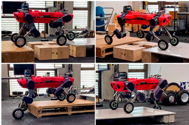
Figure 14. Our quadrupedal robot ANYmal with wheels overcomes stepping stones (upper images) and steps up-and-down (lower images) through the sampling and optimization-based approach. All motions are statically stable, that is, the robot only lifts one leg at a time.
