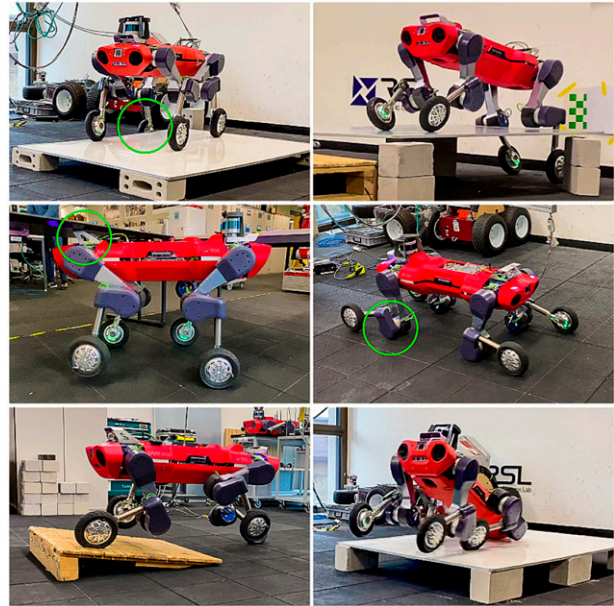
Figure 10. Recovery of the online MPC to unforeseen events. In all situations, the MPC could successfully recover and finish the executed offline trajectories. Top-left image: The motion designer did not correctly model the platform’s width, and as such, the robot’s front-left leg fell from the platform. Top-right image: While stepping up two steps, the end-effector moved the top platform since it was not properly secured. Due to this misalignment of the terrain, the front legs fell from the platform. Middle-left image: The front part of the torso hit the table while executing a dynamic 90°turn. Middle-right image: The hind legs’ knee protectors collided with the ground during a ducking motion since the offline trajectory did not consider the protector’s collision model. Lower-left image: The robot faced an unmodeled disturbance (wooden incline) on the ground while executing an offline trajectory assuming flat terrain. Lower-right image: The snapshot shows a time instance when the hind legs overcome the step. Here, the front legs slipped on the platform, and the front part of the torso collided with the platform.
