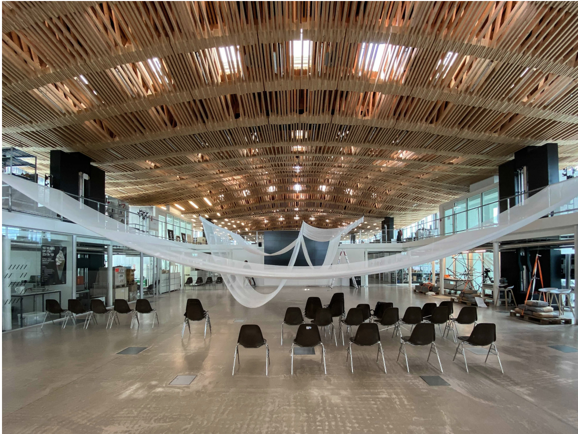
Figure 7. Physical suspension mock-up of different fabric materials. The analysis of diverse physical models allowed finding the desired balance between weight and translucency of the fabric. Photo by Shuaizhong Wang.
