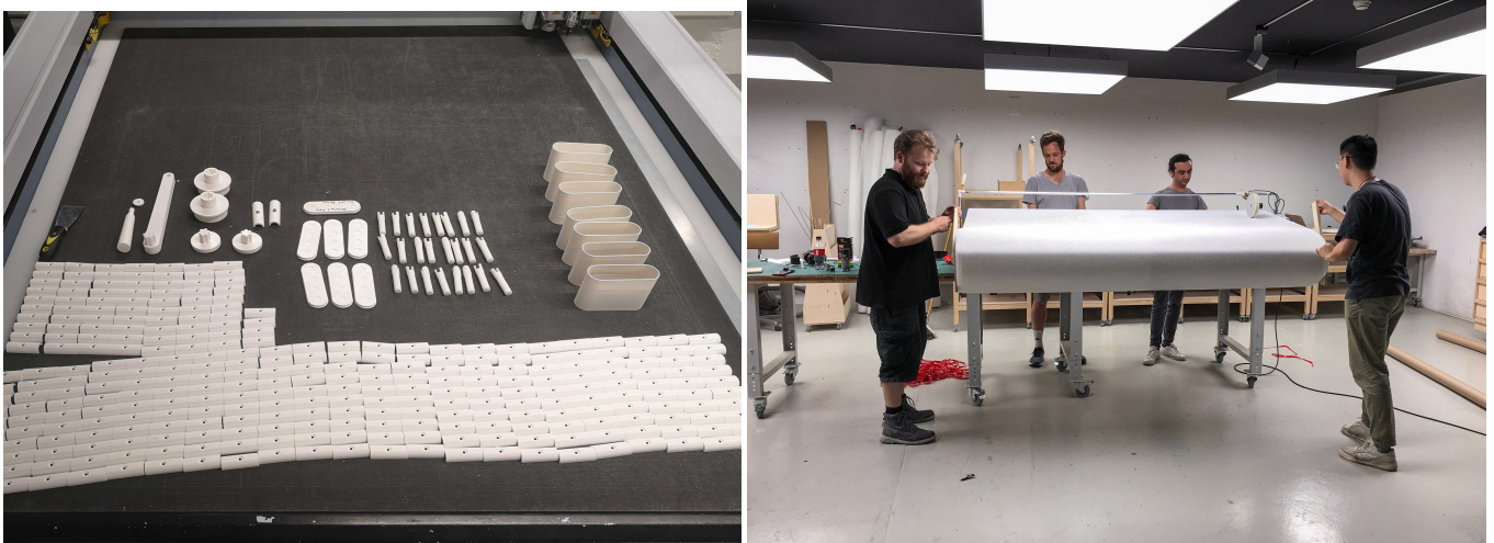
Figure 14. (a) The 3D-printed and laser-cut elements for the joints (Photo by Alessandro Tellini); (b) The rolling machine for measuring the fabric strips and for the installation of the pipes developed at the Raplab (ETH Zurich) (Photo by Giulia Boller).
