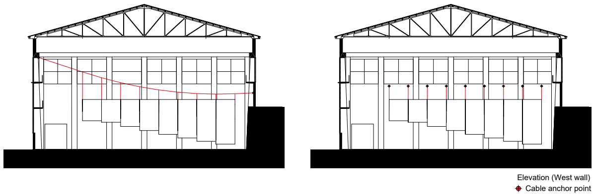
Figure 8. (a) Spanning the cables along the short side of the building would have called for a secondary structure to keep the top part of the fabric strips on the same height; (b) Conversely, when the cables span the longitudinal direction, it is possible to avoid the need for this secondary structure.
