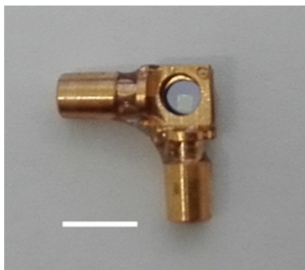
Figure 3.4. Optical Micrograph of the 2-Pin Sample Holder. To facilitate the acquisition of images at two sample-relative polarization states, we constructed a simple 2-pin sample holder, as shown above. The holder was created by fixing two OMNY sample holder pins (Membrane Type) at \sim 90 degrees to each other. The silicon nitride membrane, carrying the sample, was then glued onto this holder. Scale bar is 5 mm. Measurements were carried out with a fixed horizontal beam polarisation, following the acquisition of the first spectral image series the sample holder was azimuthally rotated to create the second polarization state with respect to the sample. Figure reproduced from [91] / CC BY-NC.
