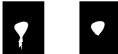
Figure 18: HSC shadowgraphy at the inlet nozzle before and after bubble breakaway from the work of Baur [105] after binarization.
