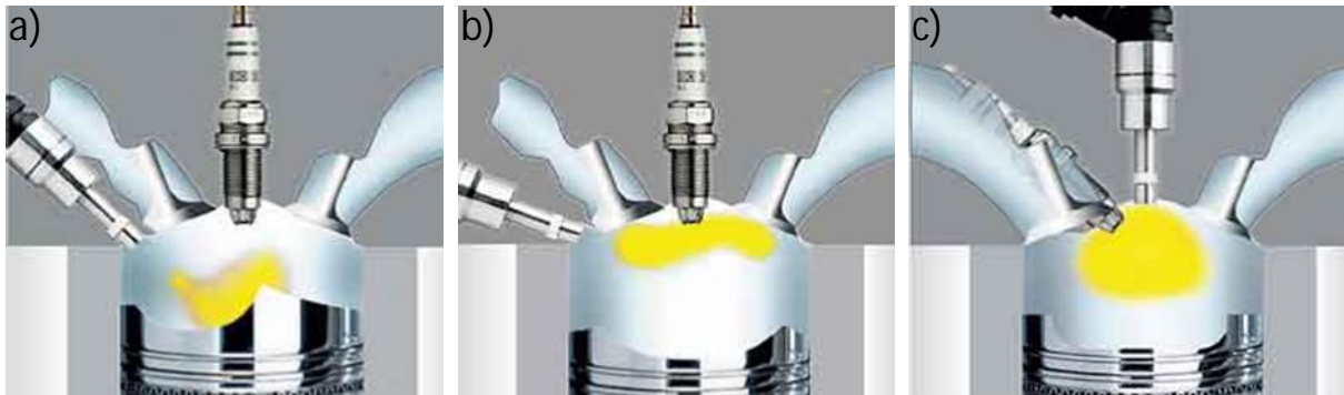
Figure 2-1 – Principle stratification applications: a) wall guided, b) air guided, c) spray guided [24]
