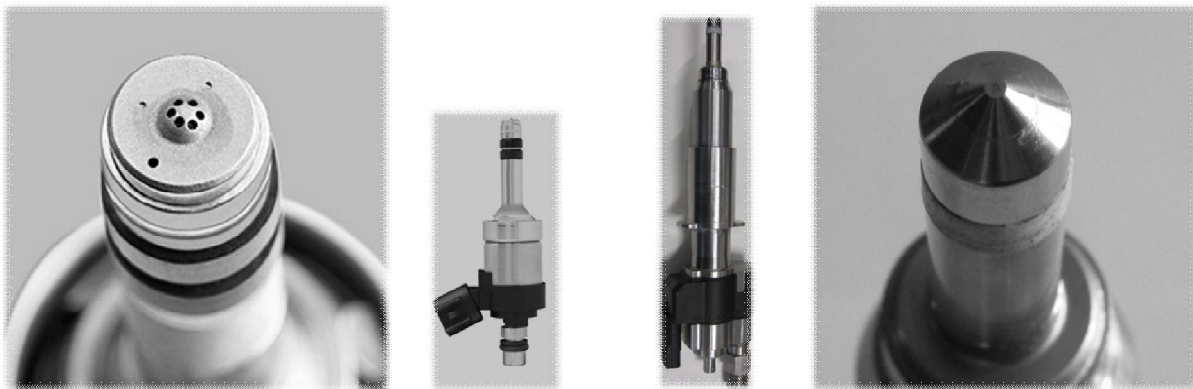
Figure 2-3 – GDI Multihole Injector (left) [32] and the Piezo hollow cone injector applied in the present work (right)
